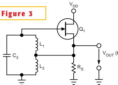
You can develop a Hartley oscillator based on a JFET transistor.
