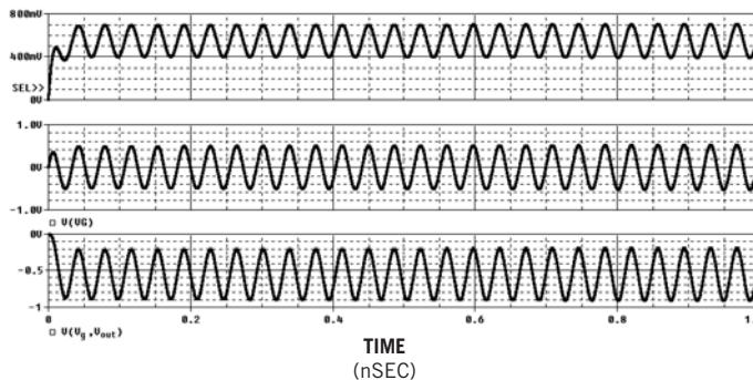
With  $C_1$  having a value of 50 nF and  $C_2$  having a value of 114 nF, the circuit oscillates.
