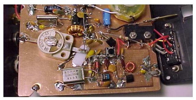
Start with a plain copper-clad board. Glue ICs down with the leads sticking up in the air. Then solder to them
