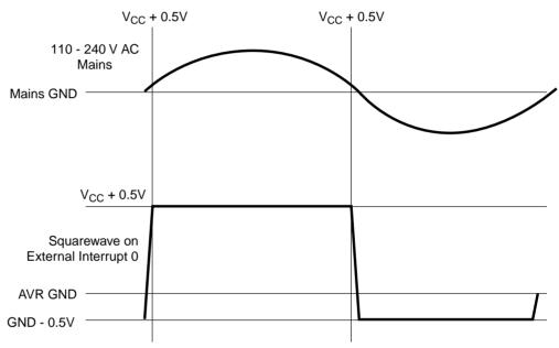
Figure 3. Oscilloscope Screenshot of Square Wave Input on External Interrupt 0-pin
