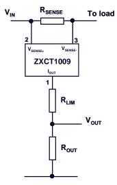
ZXCT1009 with additional current limiting Resistor R<sub>LIM</sub>.
