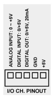
The IO-204 module has 4 for these ports on the front edge labeled "I/O CHANNELS". All of the channels can be controlled independent from one another. Furthermore, all of the function pins within a single channel can be controlled individually. The only property that is shared among all the function pins on a particular channel is the "method of data push" (see section 5.3.3)
