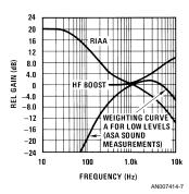
FIGURE 6. Relative Gain for RIAA, ASA Weighting A, and H-F Boost Curves
