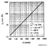
FIGURE 4. Thermal Noise of Resistor
