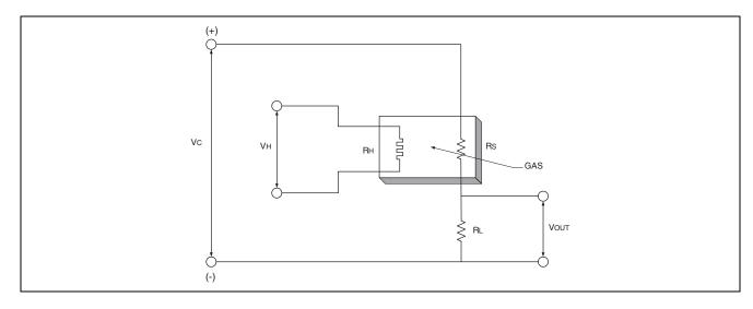
Figure 2 Sample Basic Measurement Circuit for the Sensor
