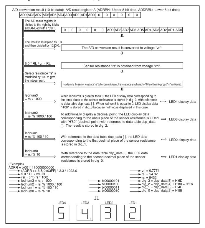
Figure 5 How the Resistance is Displayed on the LEDs
