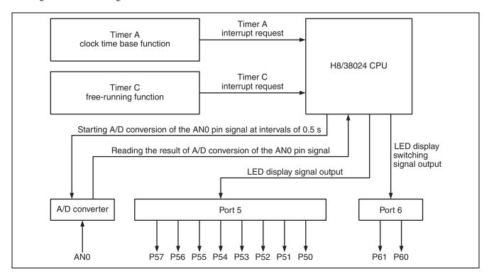
Figure 6 Block Diagram of Functions Used in This Sample Task
