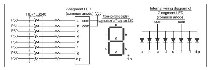
Figure 7 Connection Diagram and Internal Connections of 7-Segment LED
