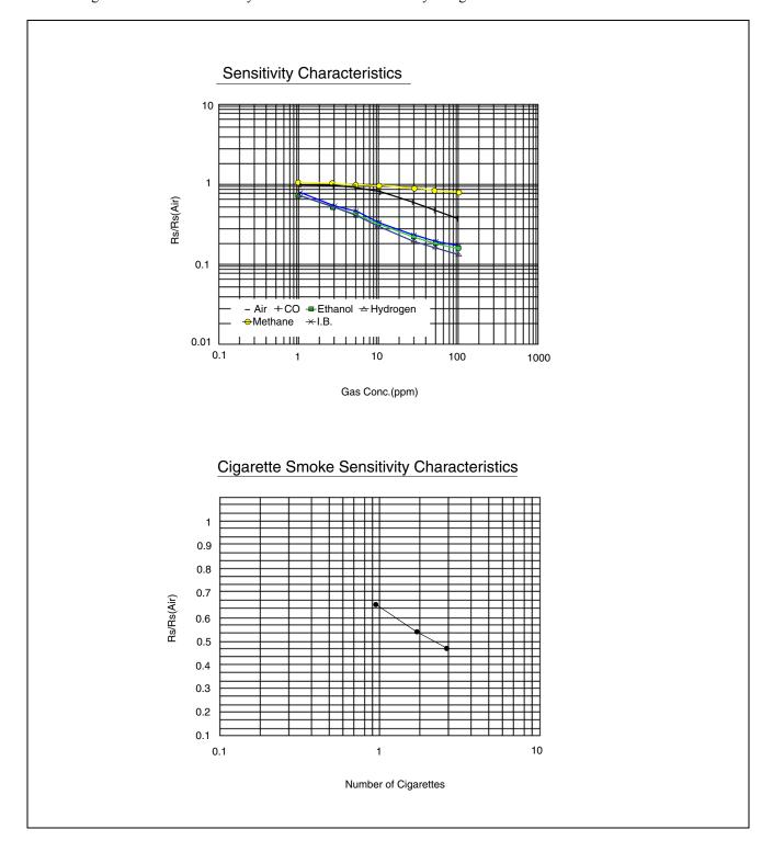
Figure 3 Sensor Sensitivity Characteristics (Reference Values)
