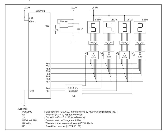
Figure 1 Hardware Configuration
