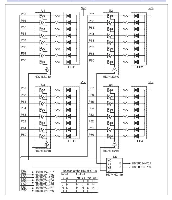
Figure 4 Method of Controlling 7-Segment LEDs
