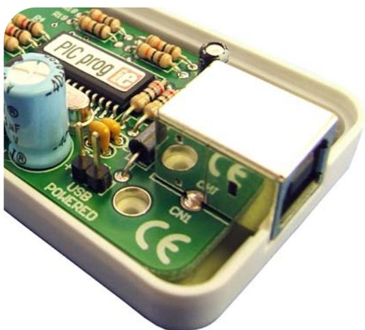
This picture shows the position of jumper when *PICflash* programmer is powered by the target board (target board have its own power supply).
