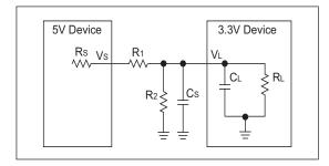
Typically, the source resistance, Rs, is very small (less than  $10\Omega$ ) so its affect on R1 will be negligible provided that R1 is chosen to be much larger than Rs. At the receive end, the load resistance, RL, is very large (greater than  $500~k\Omega$ ) so its affect on R2 will be negligible provided that R2 is chosen to be much less than RL.
