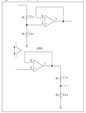
If the resistor divider is before the unity gain follower, then the lowest possible impedance is provided for the 3.3V circuits. Also, the op amp can be powered from 3.3V, saving some power. If the X is made very large, then power consumed by the 5V side can be minimized.
