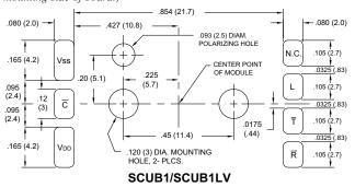
Note: All hole size tolerances ±0.003" (0.08 mm) All other tolerances ±0.005" (0.13 mm)
