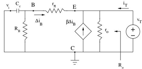
$$\text{KCL: } i_T = -\Delta i_B + \frac{v_T}{r_o} - \beta \Delta i_B$$
