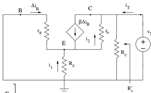
where we have used  $r_\pi/\beta = r_e$ . Generally  $r_o \gg r_e$  (first approximation below) and for most circuit,  $R_E \ll r_\pi$  (second approximation) leading to
