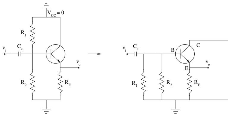
We can combine  $R_1$  and  $R_2$  into  $R_B$  (same resistance that we encountered in the biasing analysis) and replace the BJT with its small signal model:
