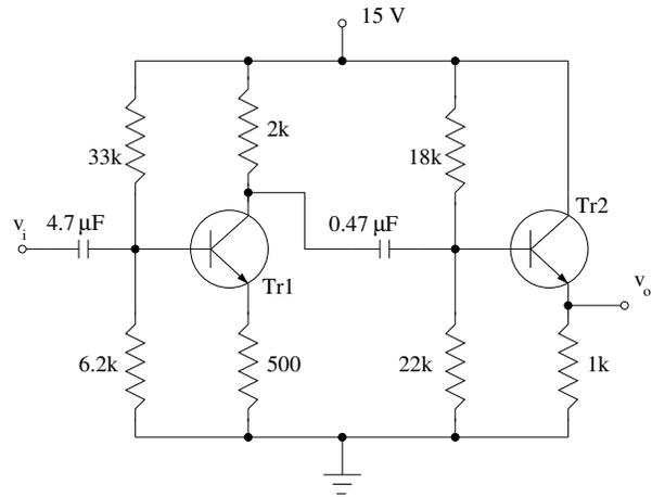
For Tr1, we replace the bias resistors (6.2k and 33k) with their Thevenin equivalent and proceed with DC analysis:
