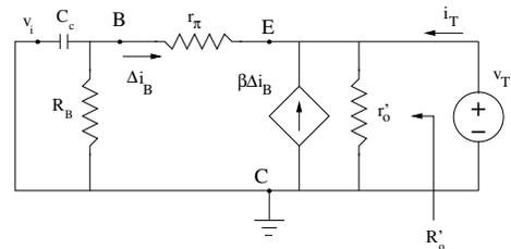
We can use our previous results by noting that we can replace  $r_o$  and  $R_E$  with  $r'_o = r_o \parallel R_E$  which results in a circuit similar to the case with no  $R_L$ . Therefore,  $R'_o$  has a similar expression as  $R_o$  if we replace  $r_o$  with  $r'_o$ :
