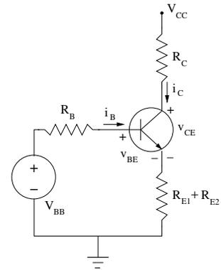
$R_1$  can be found by dividing the two equations:  $R_1 = 50 \text{ k}\Omega$  and  $R_2$  is found from the equation for  $V_{BB}$  to be  $R_2 = 3.6 \text{ k}\Omega$ . Commercial values are  $R_1 = 51 \text{ k}\Omega$  and  $R_2 = 3.6 \text{ k}\Omega$
