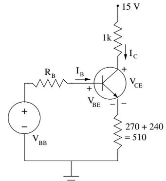
AC analysis: The circuit is a common collector amplifier with an emitter resistance. Note that the  $240 \text{ }\Omega$  resistor is shorted out with the by-pass capacitor. It only enters the formula for the lower cut-off frequency. Using the formulas in page 134 (with  $R_{E1} = 270 \text{ }\Omega$ ):
