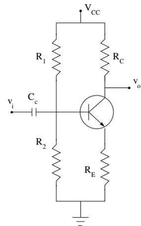
Values of  $R_C$  and  $R_E$  can be found from the above equation together with the AC gain of the amplifier  $A_V = 10$ . Ignoring  $r_e$  compared to  $R_E$  (usually a good approximation), we get:
