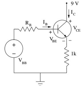
AC analysis: The circuit is a common collector amplifier. Using the formulas in page 134,
