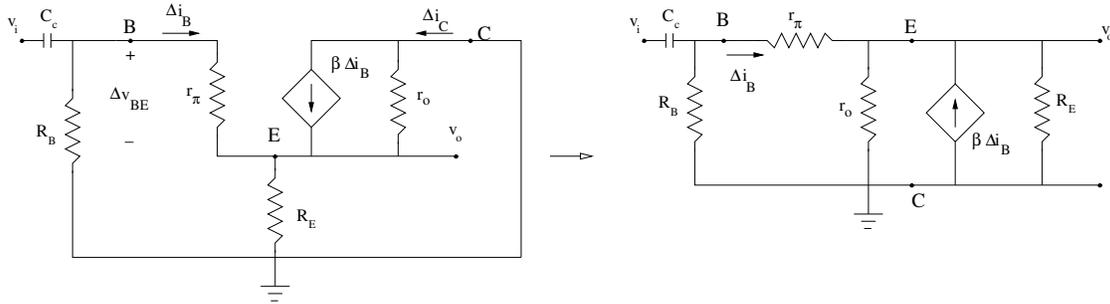
The figure above shows why this is a common collector configuration: collector is shared between input and output AC signals. We can now proceed with the analysis. Node voltage method is usually the best approach to solve these circuits. For example, the above circuit will have only one node equation for node at point E with a voltage  $v_o$ :
