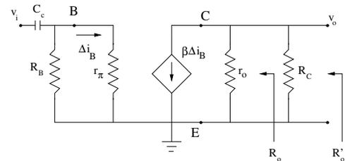
The negative sign in  $A_v$  indicates  $180^\circ$  phase shift between input and output. The circuit has a large voltage gain but has a medium value for input resistance.
