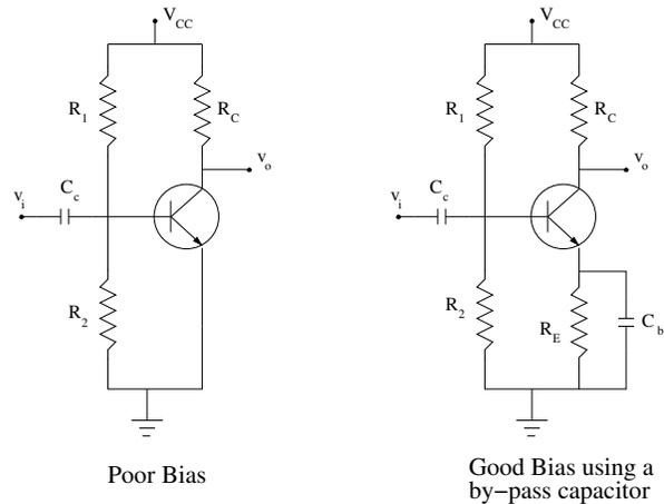
For this new circuit and with the capacitors open circuit, this circuit is the same as our good biasing circuit of page 110. The bias point currents and voltages can be found using procedure of pages 110-112.
