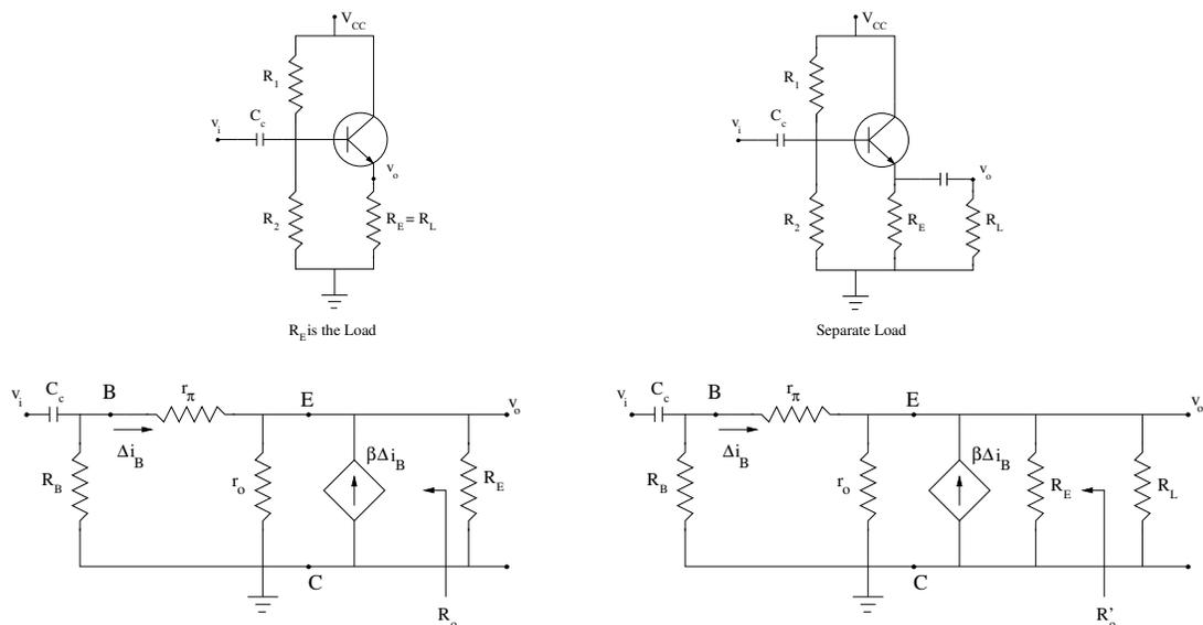
Alternatively, the load can be placed in parallel to  $R_E$ . This is done when the common collector amplifier is used as a buffer ( $A_v \approx 1$ ,  $R_i$  large). In this case, the output resistance is denoted by  $R'_o$  (see figure). For this circuit, BJT sees a resistance of  $R_E \parallel R_L$ . Obviously, if we want the load not to affect the emitter follower circuit, we should use  $R_L$  to be much
