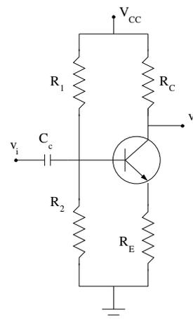
$$\frac{v_E - v_i}{r_\pi} + \frac{v_E}{R_E} - \beta\Delta i_B + \frac{v_E - v_o}{r_o} = 0$$
