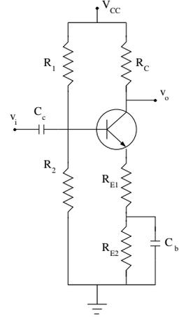
The addition of by-pass capacitor, however, modifies the lower cut-off frequency of the circuit. Similar to a regular common emitter amplifier with no emitter resistance, both the coupling and bypass capacitors contribute to setting the lower cut-off frequency for this amplifier. Similarly we find that an approximate formula for the cut-off frequency (accurate within a factor of two and exact at the limits) is:
