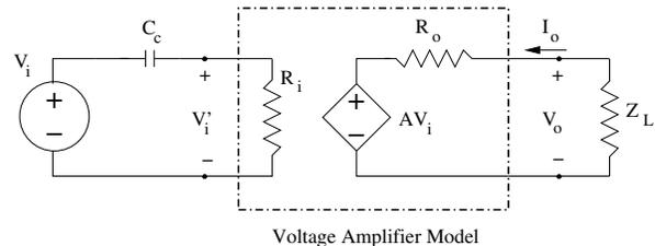
When we account for impedance of the capacitor, we have set up a high pass filter in the input part of the circuit (combination of the coupling capacitor and the input resistance of the amplifier). This combination introduces a lower cut-off frequency for our amplifier which is the same as the cut-off frequency of the high-pass filter:
