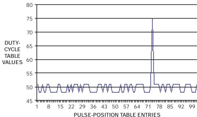
**Figure 4** Devised for testing a serial link's error response, this waveform plot displays pulses' locations within the waveform (horizontal axis) versus the duty cycle for each pulse (vertical axis). The waveform cycle repeats after pulse 100 ends.
