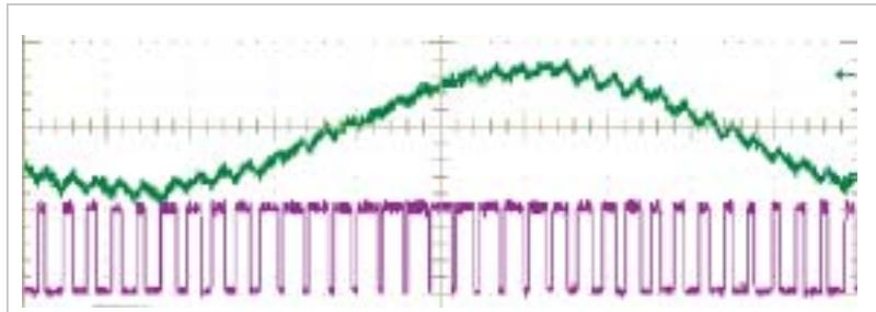
**Figure 3** After undergoing lowpass-filtering, the controller's pulse-width-modulated output (lower trace) reveals its sine-wave origin.
