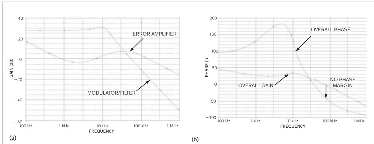
Figure 3 Gain (a) and phase (b) plots show that using a ceramic-dielectric output-filter capacitor erodes the phase-angle margin and pushes the circuit dangerously close to oscillation.
