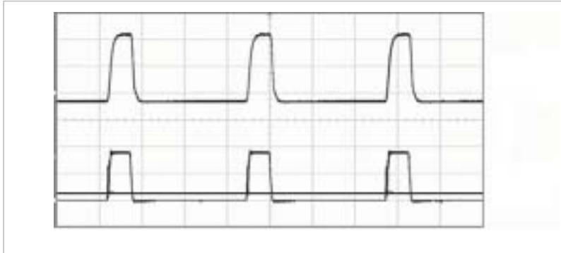
**Figure 2** For a 3V-dc input (lower trace, horizontal line), the voltage at regulator IC<sub>1</sub>'s SW pin reaches a peak of approximately 18V (lower trace, pulsed waveform). The 1-to-6 step-up turns ratio of inductor L<sub>1</sub> further increases the peak output voltage to 160V (upper trace) to produce 100V dc. The upper trace's lower limit goes to  $-6 \times V_{IN} (-18V)$  due to the tapped inductor.
