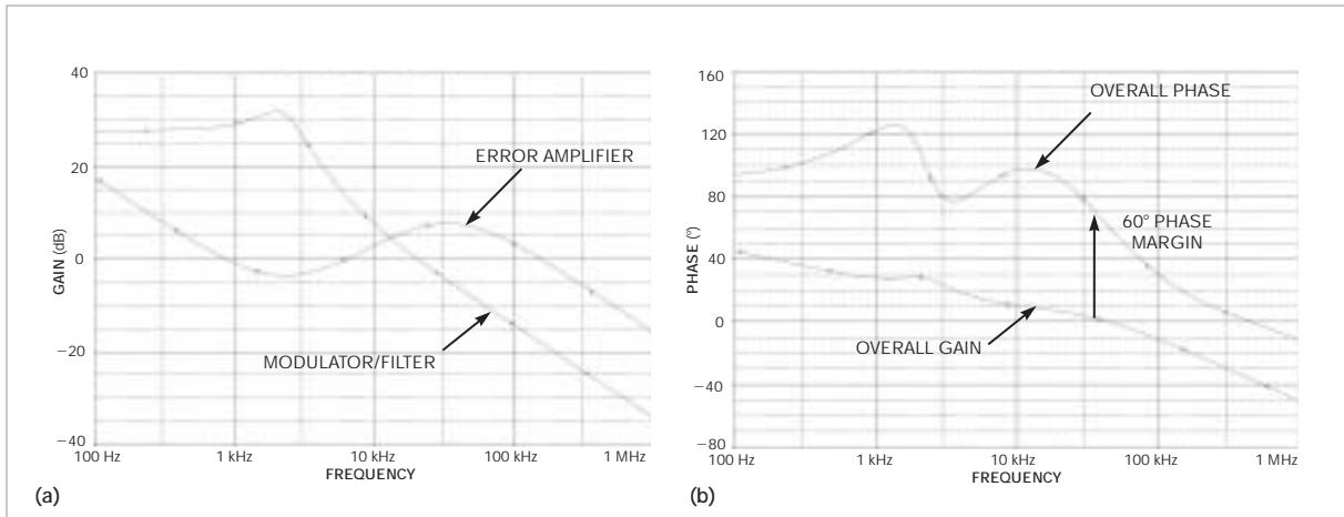
Figure 2 Gain (a) and phase (b) plots show that the circuit of Figure 1a includes adequate compensation and phase-angle margin for an aluminum electrolytic output-filter capacitor.
