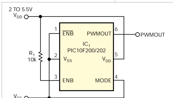
**Figure 1** A microcontroller and a resistor can deliver a complex PWM output.
