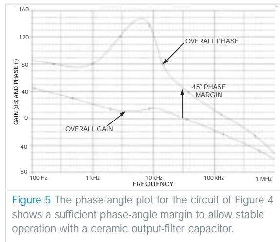
Figure 5 The phase-angle plot for the circuit of Figure 4 shows a sufficient phase-angle margin to allow stable operation with a ceramic output-filter capacitor.
