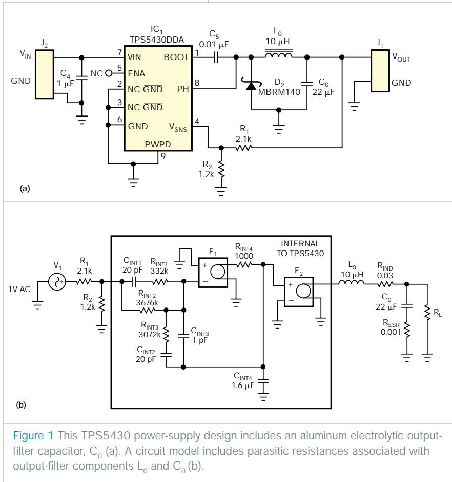
**Figure 1** This TPS5430 power-supply design includes an aluminum electrolytic output-filter capacitor,  $C_0$  (a). A circuit model includes parasitic resistances associated with output-filter components  $L_0$  and  $C_0$  (b).
