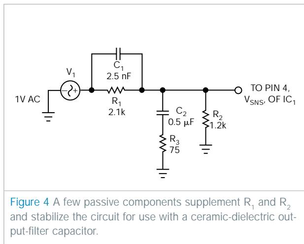
Figure 4 A few passive components supplement  $R_1$  and  $R_2$  and stabilize the circuit for use with a ceramic-dielectric output-filter capacitor.
