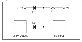
When output voltage specifications are determined, it is done assuming that the output is driving a load between the output and ground for the high output, and a load between 3.3V and the output for the low output. If the load for the high threshold is actually between the output and 3.3V, then the output voltage is actually much higher as the load resistor is the mechanism that is pulling the output up, instead of the output transistor.
