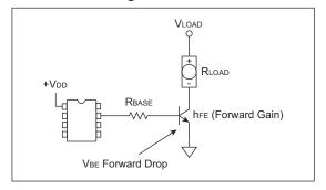
The value of RBASE will depend on the microcontroller supply voltage. Equation 18-1 describes how to calculate RBASE.
