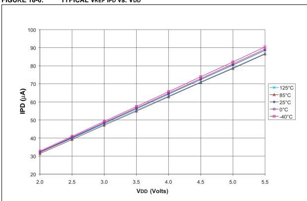
FIGURE 18-6: TYPICAL VREF IPD vs. VDD
