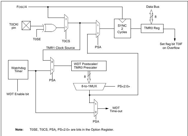
FIGURE 6-1: BLOCK DIAGRAM OF THE TIMER0/WDT
