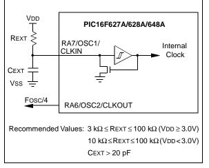
The RC Oscillator mode has two options that control the unused OSC2 pin. The first allows it to be used as a general purpose I/O port. The other configures the pin as an output providing the Fosc signal (internal clock divided by 4) for test or external synchronization purposes.
