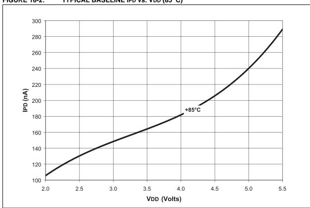
FIGURE 18-2: TYPICAL BASELINE IPD vs. VDD (85°C)
