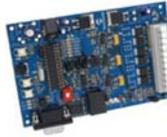
This board offers a cost-effective method of evaluating and developing sensed or sensorless brushless DC (BLDC) motor control applications. The board supports 28-pin, PIC18 microcontrollers and is capable of controlling motors rated up to 48V and 2.2 amps. Pre-programmed PIC18F2431 and dsPIC30F3010 devices are included.
