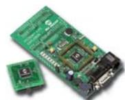
This low-cost demo board is used to evaluate the performance of High Pin Count (HPC) 8-bit PIC18F series microcontrollers. The board features a PIC18F8722, which is the superset of the entire 64 and 80-pin PIC18F general purpose family. A daughter board (mezzanine) is also part of the kit and allows different processors sharing the same pin-out to be mounted and tested on the Explorer board.
