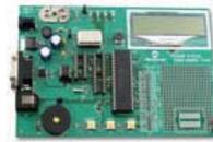
The PICDEM 2 Plus demonstrates the capabilities of the 18, 28 and 40-pin PIC18 and PIC16 devices. It can be used stand-alone with a programmed part and with MPLAB REAL ICE or MPLAB ICD 2. The board has a
