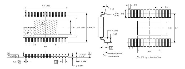
For reference only (reference JEDEC MO-153 AET) Dimensions in millimeters
