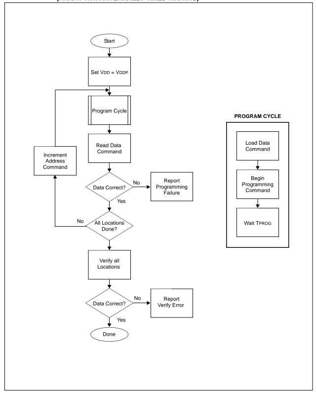
For PIC18 devices, an erase must be done separately before a write. Special commands that are triggered by writing to the configuration test area are used to clear blocks of program memory, the entire program memory, the configuration words, the data EEPROM or the entire device.
