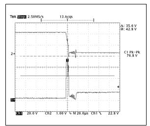
FIGURE 5: Inductive kick voltage spike. No slow down capacitor, 20 µs time scale.
