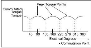
**FIGURE 2:** BDC Fan Torque Characteristics (Fan Running Continuously).
