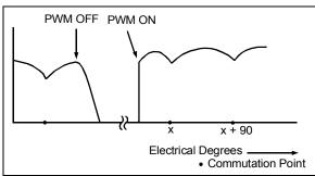
FIGURE 3: BDC Fan Torque Characteristics (PWM Control).
