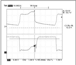
**FIGURE 7:** Using a 10  $\mu$ F slow down capacitor with 1.1 k $\Omega$  base resistor. Notice the lack of voltage spike and more rounded edges of Trace 1.
