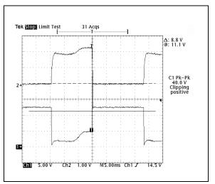
FIGURE 6: Inductive kick voltage spike. No slow down capacitor, 5 ms time scale.
