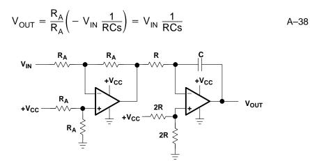
Figure A–33. Noninverting Integrator with Inverting Buffer
