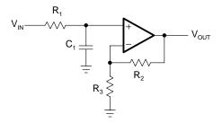
Figure 16–12. First-Order Noninverting Low-Pass Filter
