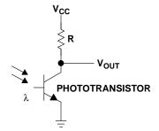
Figure 12–9. Phototransistor Amplifier
