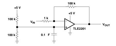
Figure 10–16. Improved TLC2201 Op Amp Circuit
