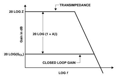
Figure 9–4. CFA Gain vs Frequency
