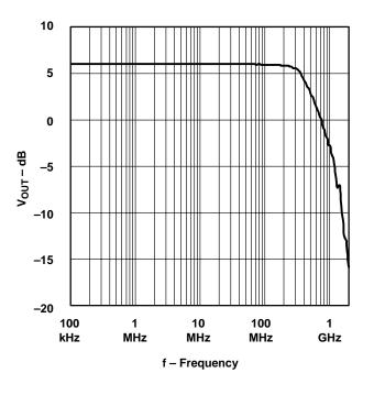
Figure 13–14. Gain vs Frequency Plot for THS3201
