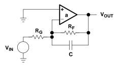
Figure 7–13. Lead-Compensation Circuit
