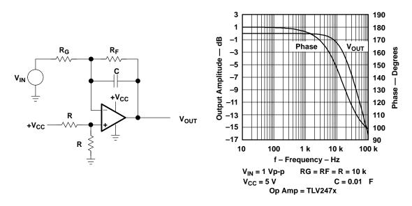
Figure A-32. Inverting Integrator with Resistive Reset
