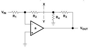
Figure 3–7. T Network in Feedback Loop
