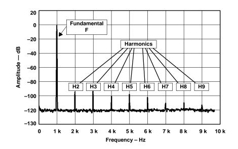
Figure 14–6. Total Harmonic Distortion
