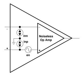
Figure 10–7. Op Amp Circuit Noise Model
