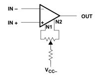
Figure 11–2. Offset Voltage Adjust
