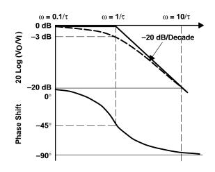
Figure 5–9. Bode Plot of Low-Pass Filter Transfer Function
