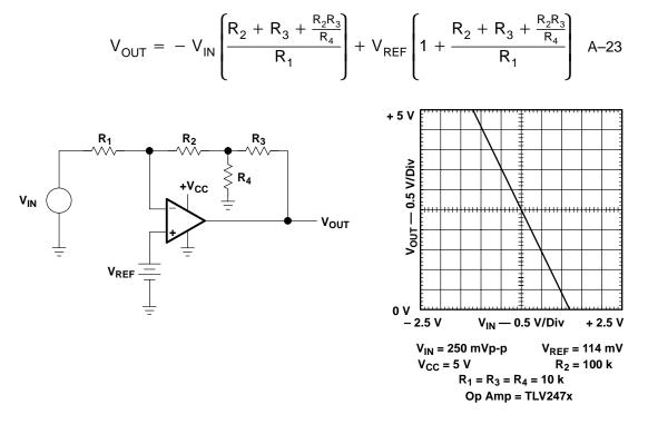
Figure A-20. T Network in the Feedback Loop
