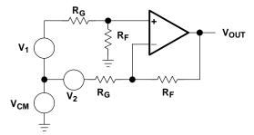
Figure 3–6. Differential Amplifier With Common-Mode Input Signal
