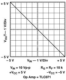
Figure A–1. Split-Supply Op Amp Circuit
