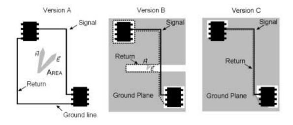
Figure 17–9. Loop and Slot Antenna Board Trace Layouts
