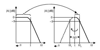
Figure 16–31. Low-Pass to Band-Pass Transition
