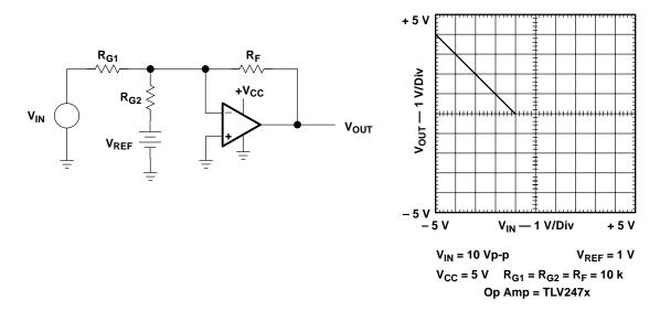
Figure A–8. Inverting Op Amp with Inverting Positive Reference
