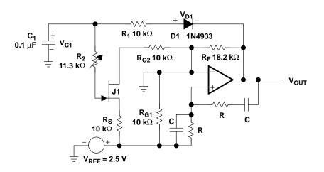
Figure 15–12. Wien Bridge Oscillator with AGC
