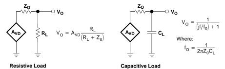
Figure 11–6. Effect of Output Impedance
