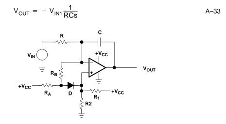
Figure A–28. Inverting Integrator with Input Current Compensation
