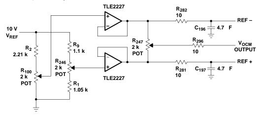
Figure 13–10. External Voltage Reference Circuit for ADC/DAC.
