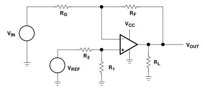
Figure 4–16. Schematic for Case 3:  $V_{OUT} = -mV_{IN} + b$
