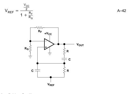
Figure A–37. Basic Wien Bridge Oscillator
