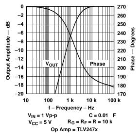
Figure A–22. Inverting AC Amplifier
