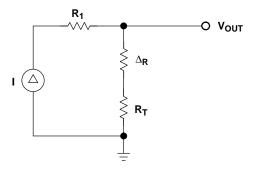
Figure 12–5. Current Source Excitation for a Resistive Transducer
