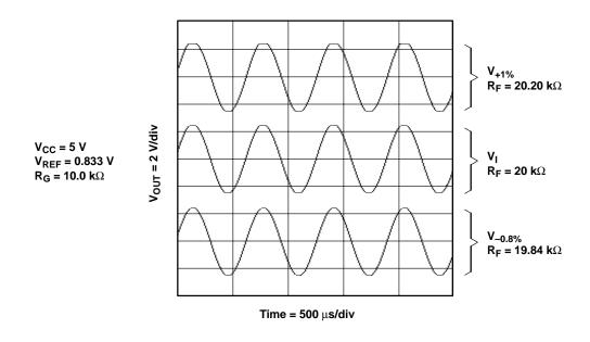
Figure 15–9. Wien Bridge Output Waveforms
