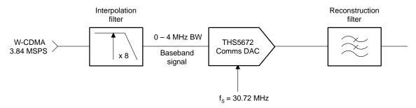
Figure 13–4. Communication DAC with Interpolation and Reconstruction Filters
