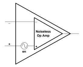
Figure 10-8. Equivalent Op Amp Circuit Noise Model
