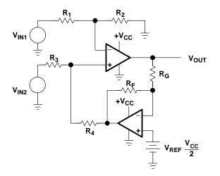
Figure A–19. Variable Gain Differential Amplifier
