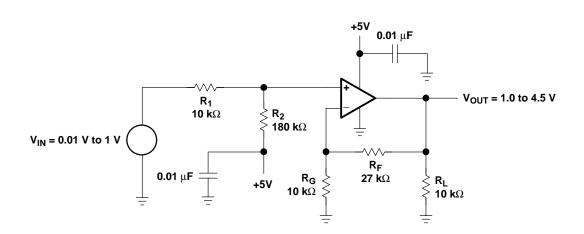
Figure 4–11. Case 1 Example Circuit
