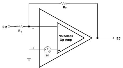
Figure 10–10. Inverting Equivalent Op Amp Circuit Noise Model
