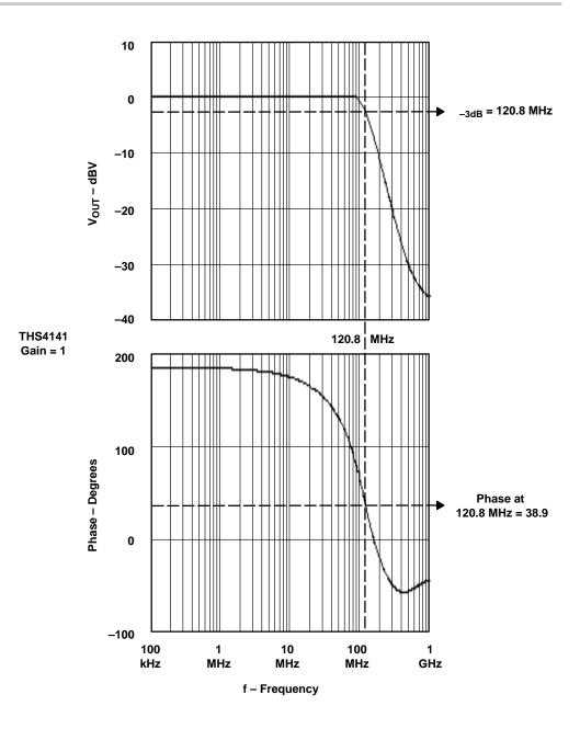
Figure 13–12. Differential Amplifier Closed-Loop Response
