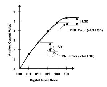
Figure 14–9. Differential Nonlinearity Error
