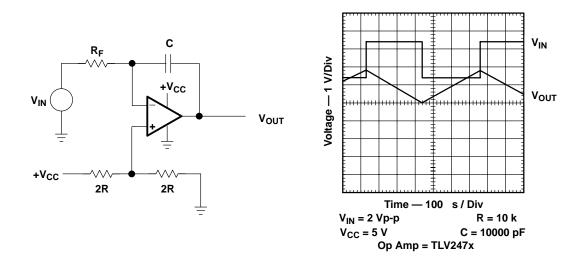
Figure A–27. Inverting Integrator
