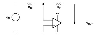
Figure 4–4. Single-Supply Op Amp Circuit
