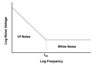
Figure 11–9. Typical Op amp Input Noise Spectrum
