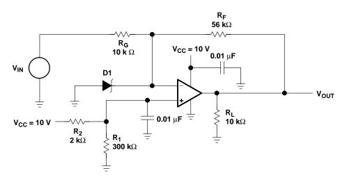
Figure 4–17. Case 3 Example Circuit
