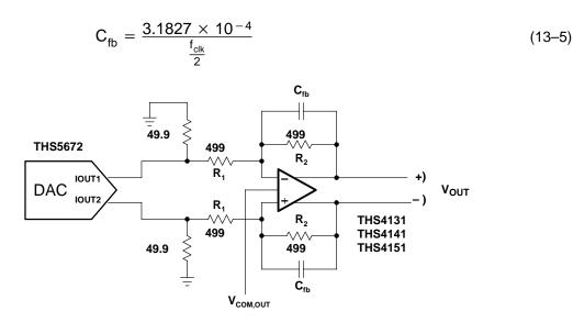
Figure 13–7. A Single-Pole Reconstruction Filter
