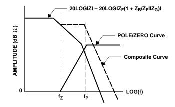
Figure 8–9. Bode Plot with C<sub>F</sub>
