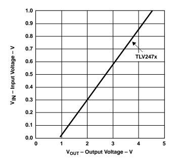
Figure 4–12. Case 1 Example Circuit Measured Transfer Curve
