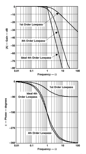
Note: Curve 1: 1st-order partial low-pass filter, Curve 2: 4th-order overall low-pass filter, Curve 3: Ideal 4th-order low-pass filter
