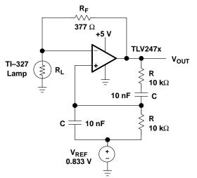
Figure 15–10. Wien Bridge Oscillator with Nonlinear Feedback
