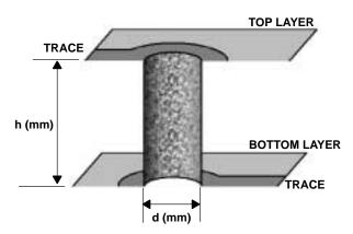
Figure 17–14. Via Inductance Measurements
