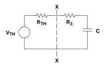
Figure 2–8. Thevenin's Equivalent Circuit for Figure 2–7
