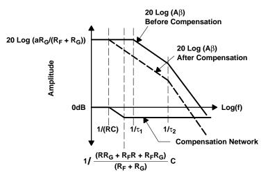
Figure 7–21. Bode Plot of Lead-Lag Compensated Op Amp
