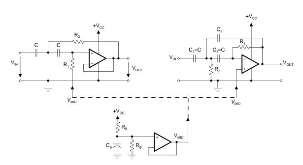
Figure 16–50. Biasing a Sallen-Key and an MFB High-Pass Filter
