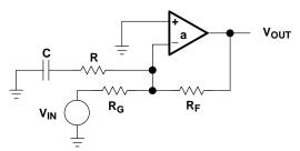
Figure 7–20. Lead-Lag Compensated Op Amp
