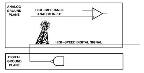
Figure 17–4. Broadcasting From PCB Traces
