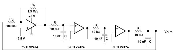
Figure 15–16. Phase Shift Oscillator, Buffered
