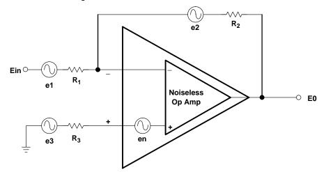
Figure 10–9. Inverting Op Amp Circuit Noise Model
