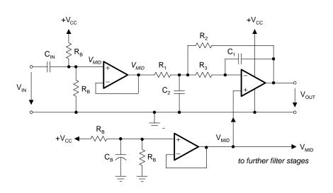
Figure 16–49. Biasing a Second-Order MFB Low-Pass Filter
