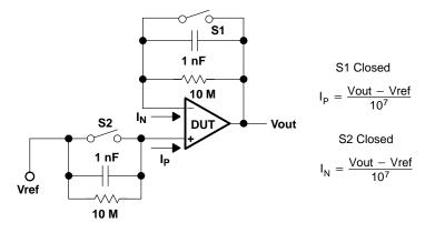
Figure 11–3. Test Circuit – I<sub>IB</sub>
