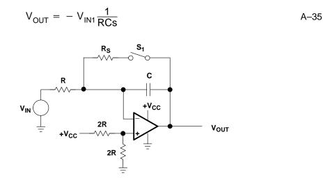
Figure A–30. Inverting Integrator with Mechanical Reset
