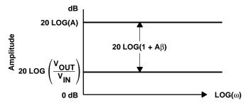
Figure 5–13. When No Pole Exists in Equation (5–12)
