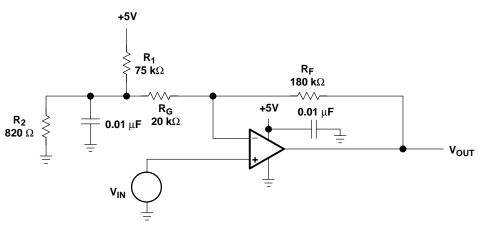
Figure 18–10. Final Schematic for the Transducer to ADC Interface Circuit
