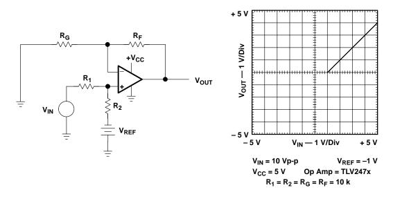
Figure A-10. Noninverting Op Amp with Noninverting Negative Reference
