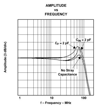
Figure 8–8. Effects of Stray Capacitance on CFAs
