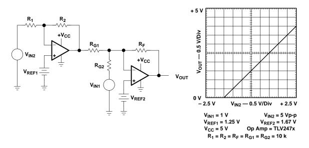
Figure A–16. High Common-Mode Range Differential Amplifier
