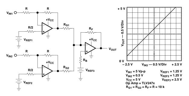
Figure A-26. Noninverting Summer with Buffers
