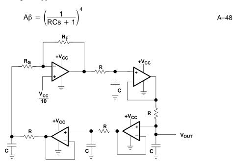
Figure A–43. Bubba Oscillator
