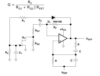
Figure A–39. Wien Bridge Oscillator with AGC
