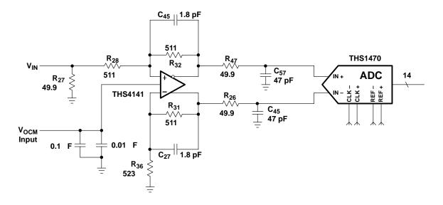
Figure 13–11. Single-Ended to Differential Output Drive Circuit
