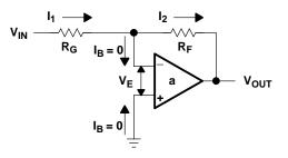
Figure 3–3. The Inverting Op Amp
