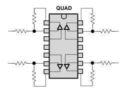
Figure 17–19. Mirror-Image Layout for Quad Op Amp Package
