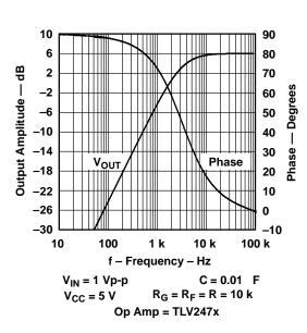
Figure A–23. Noninverting AC Amplifier
