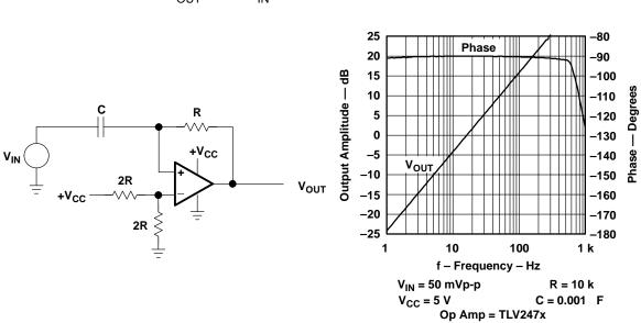
$$V_{OUT} = -V_{IN} RCs$$
