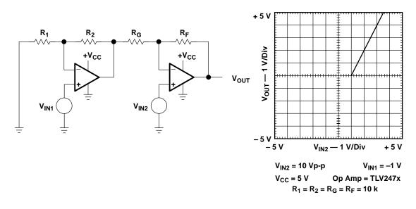
Figure A–15. High Input Impedance Differential Amplifier
