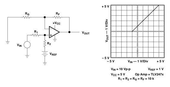
Figure A–12. Noninverting Op Amp with Noninverting Positive Reference
