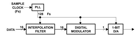
Figure 14–5. Sigma Delta D/A Converter
