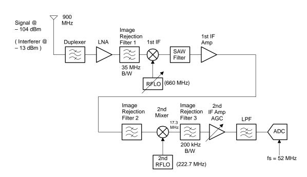
Figure 13–1. A Typical GSM Cellular Base Station Receiver Block Diagram
