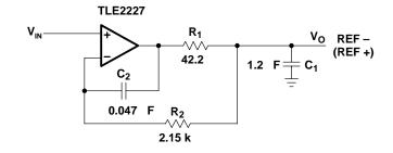
Figure 13–8. Voltage Reference Filter Circuit
