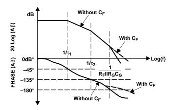
Figure 7–19. Compensated Attenuator Bode Plot
