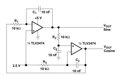
Figure 15–20. Quadrature Oscillator
