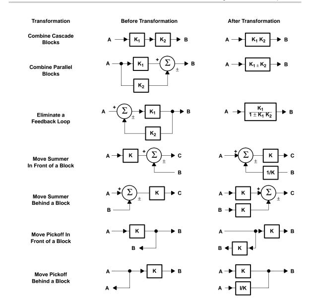
Figure 5–6. Block Diagram Transforms
