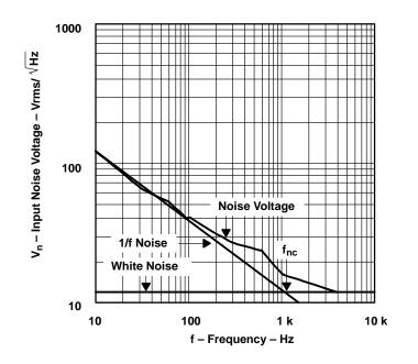
Figure 10–6. TLV2772 Op Amp Noise Characteristics
