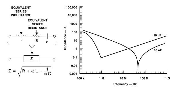
Figure 17–16. Capacitor Self Resonance
