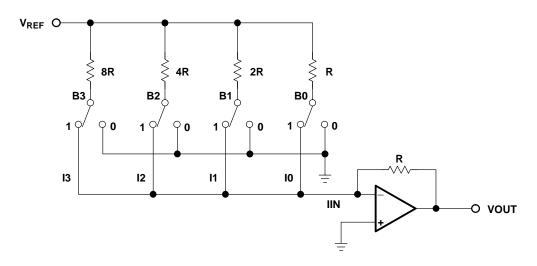
Figure 14-2. Binary Weighted D/A Converter
