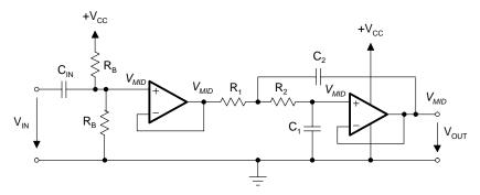
Figure 16–48. Biasing a Sallen-Key Low-Pass
