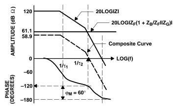
Figure 8–6. Bode Plot of Stability Equation
