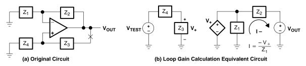
Figure 15–6. Amplifier with Positive and Negative Feedback
