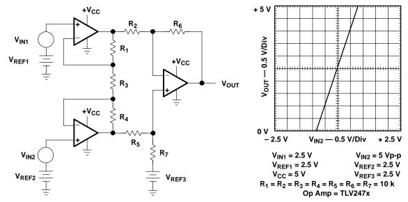
Figure A-17. High-Precision Differential Amplifier
