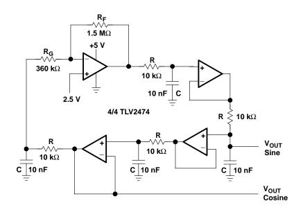
Figure 15–18. Bubba Oscillator
