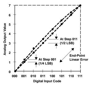
Figure 14–10. Integral Nonlinearity Error
