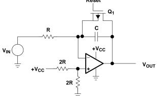
Figure A–31. Inverting Integrator with Electronic Reset
