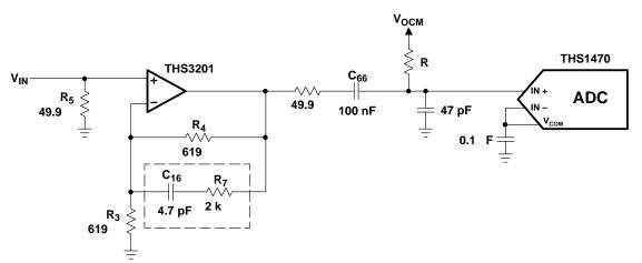
bandwidth and the frequency response shape as well as defining the gain of the circuit. R4 and R3 cannot be arbitrary values.
