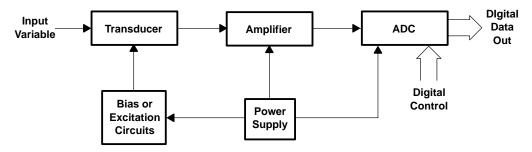
Figure 12–1. Block Diagram of a Transducer Measurement System
