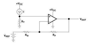
Figure 18–12. DAC Current Source to Actuator Interface Circuit
