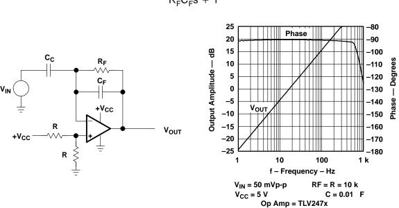
$$V_{OUT} = -V_{IN} \frac{R_F Cs}{R_F C - s + 1}$$
