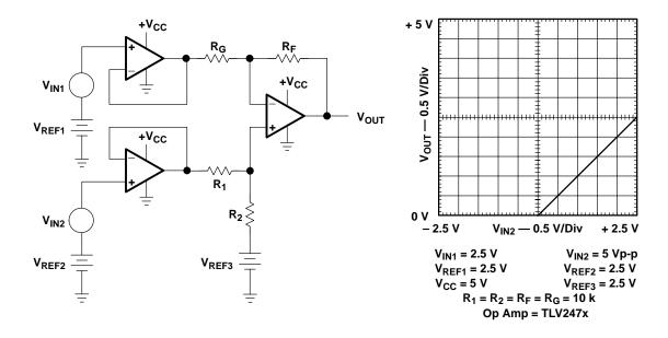
Figure A–18. Simplified High-Precision Differential Amplifier
