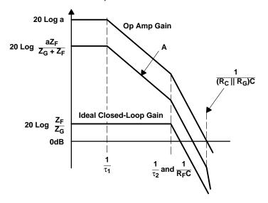
Figure 7–15. Inverting Op Amp With Lead Compensation
