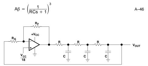
Figure A–41. Classical Phase Shift Oscillator
