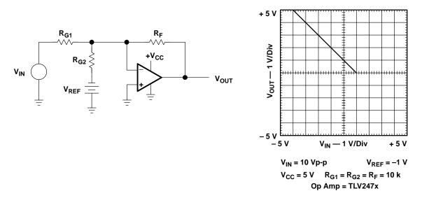
Figure A–6. Inverting Op Amp with Inverting Negative Reference
