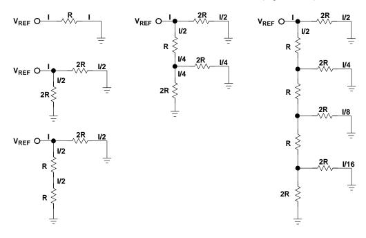
An R/R2 network can be used to make a D/A converter (Figure 14–3).
