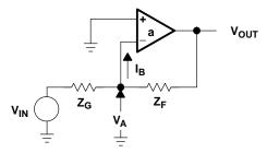
Figure 6–5. Inverting Op Amp
