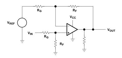
Figure 4-8. Noninverting Op Amp
