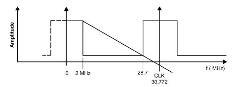
Figure 13–6. Reconstruction Filter Characteristics
