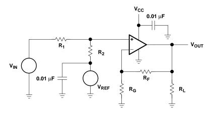
Figure 4–10. Schematic for Case1:  $V_{OUT} = +mV_{IN} + b$
