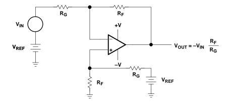
Figure 4–3. Split-Supply Op Amp Circuit With Common-Mode Voltage
