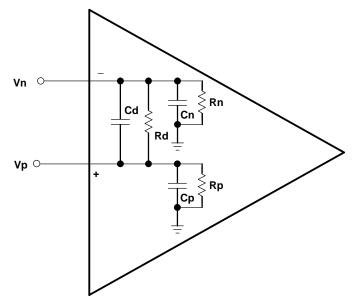
Figure 11–5. Input Parasitic Elements
