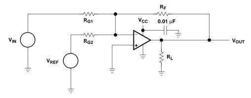
Figure 4–19. Schematic for Case 4:  $V_{OUT} = -mV_{IN} - b$
