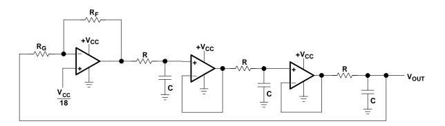
Figure A–42. Buffered Phase Shift Oscillator
