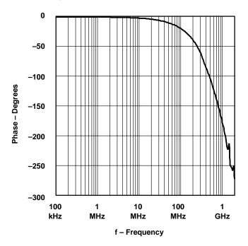
Figure 13–15. Phase vs Frequency for THS3201
