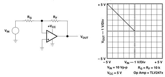
Figure A-4. Single-Supply Op Amp Circuit
