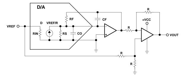
Figure 14–19. Single-Supply DAC Operation
