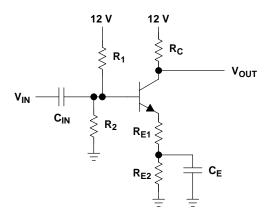
Figure 2–15. Transistor Amplifier
