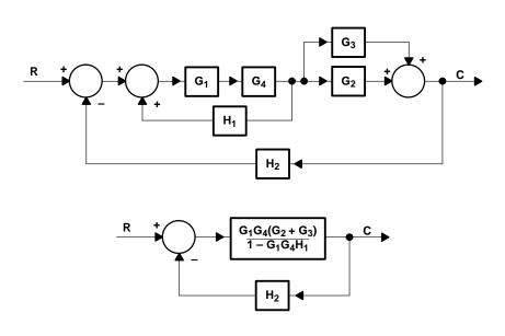
Figure 5–5. Multiloop Feedback System
