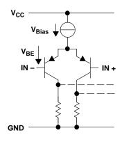
Figure 18–3. Input Circuit of a NonRRI Op Amp
