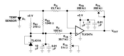
Figure 12–14. Final Analog Interface Circuit
