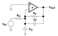
Figure 7–18. Compensated Attenuator Circuit
