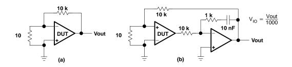
Figure 11–1. Test Circuits for Input Offset Voltage
