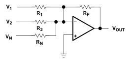
Figure 3–4. The Adder Circuit
