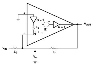
Figure 8–5. Inverting CFA
