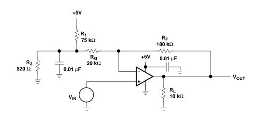
Figure 4–14. Case 2 Example Circuit
