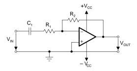
Figure 16–46. Dual-Supply Filter Circuit
