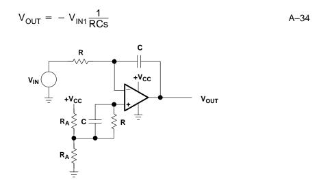
Figure A–29. Inverting Integrator with Drift Compensation
