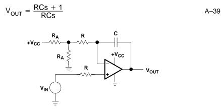
Figure A–34. Noninverting Integrator Approximation
