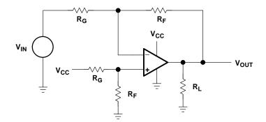
Figure 4–6. Inverting Op Amp With V<sub>CC</sub> Bias
