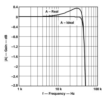
Figure 16–52. Modification of the Intended Butterworth Response to a Tschebyscheff-Type Characteristic
