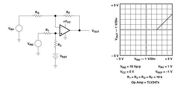
Figure A-14. Differential Amplifier with Bias Correction
