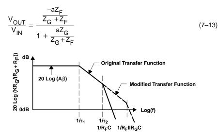
Figure 7–14. Lead-Compensation Bode Plot
