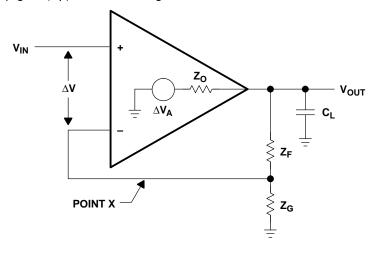
Figure 7–8. Capacitively-Loaded Op Amp
