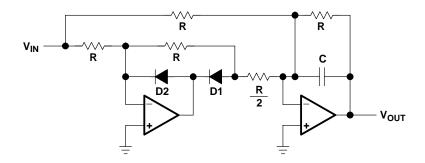
Figure 12–11. Active Full-Wave Rectifier and Filter
