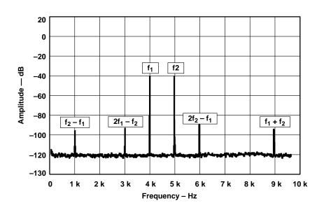
Figure 14–12. Intermodulation Distortion
