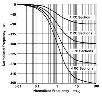
Figure 15–2. Phase Plot of RC Sections
