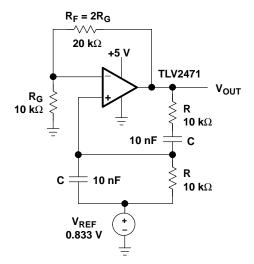
Figure 15–8. Final Wien Bridge Oscillator Circuit
