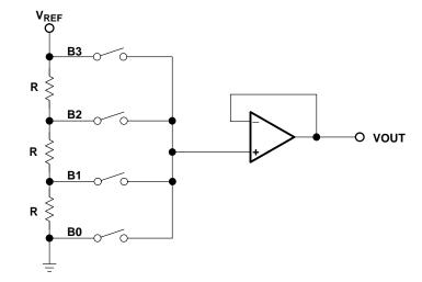
Figure 14–1. Resistor Ladder D/A Converter
