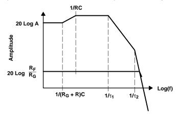
Figure 7–22. Closed-Loop Plot of Lead-Lag Compensated Op Amp
