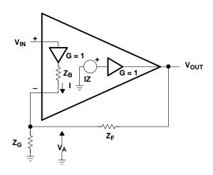
Figure 8-4. Noninverting CFA
