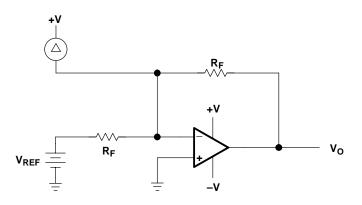
Figure 18–13. DAC Current Sink to Actuator Interface Circuit
