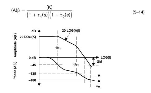
Figure 5–15. Magnitude and Phase Plot of Equation 5–14
