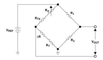
Figure 12–7. Wheatstone Bridge Circuit
