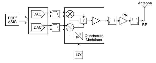
of the DAC, is usually a high-order Bessel or elliptic filter used to low-pass filter the analog output from the DAC.
