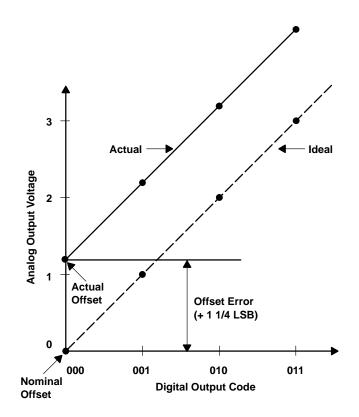
Figure 14–7. D/A Offset Error
