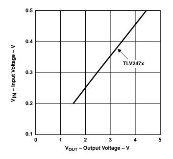
Figure 4–15. Case 2 Example Circuit Measured Transfer Curve
