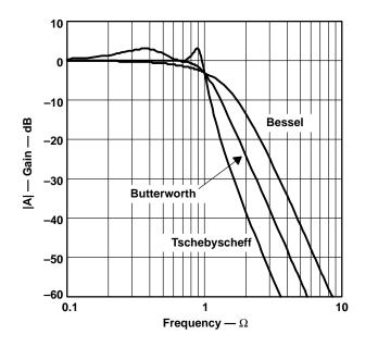
Figure 16–9. Comparison of Gain Responses of Fourth-Order Low-Pass Filters
