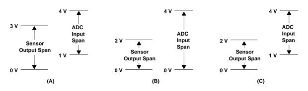
Figure 12–3. Example of Spans That Require Correction
