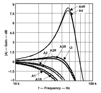
The difference between ideal and real response peaks with 0.35 dB at approximately 30 kHz, which is equivalent to an enormous 4.1% gain error can be seen.
