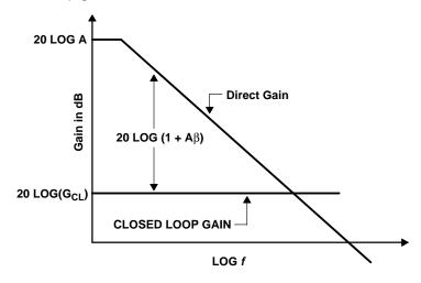
Figure 9–3. VFA Gain versus Frequency
