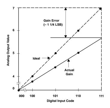
Figure 14–8. D/A Gain Error
