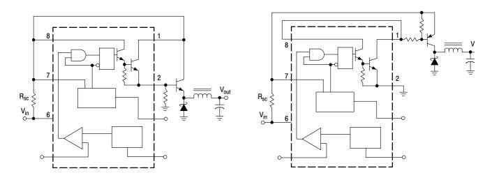
Figure 11. External Current Boost Connections for I<sub>C</sub> Peak Greater than 1.5 A
