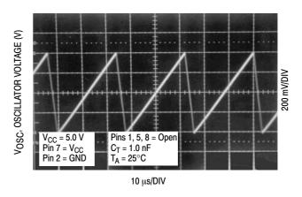
**Figure 3. Timing Capacitor Waveform**
