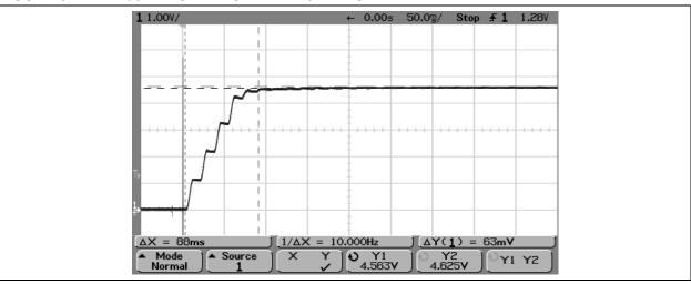
FIGURE 7: Vout AT START-UP WITH 270 $\Omega$  LOAD
