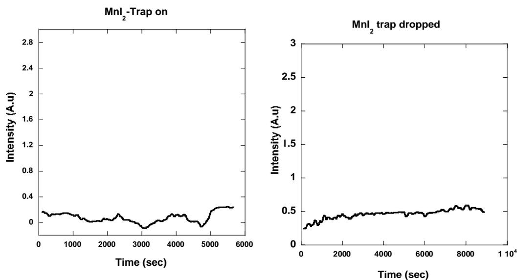
TPD (temperature-program desorption) was performed by trapping gases from heated MnI<sub>2</sub> using a cold trap and then dropping the trap to evaporate the condensed gas.
