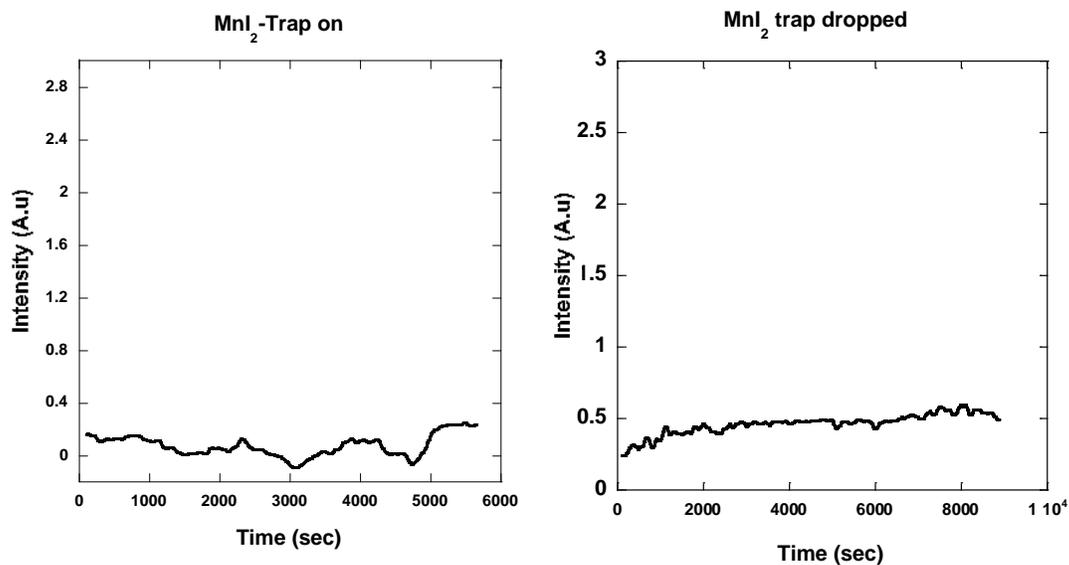
Trapping gases from heated MnI<sub>2</sub> using a cold trap and then dropping the trap to evaporate the condensed gas by use of TPD (temperature-program desorption)
