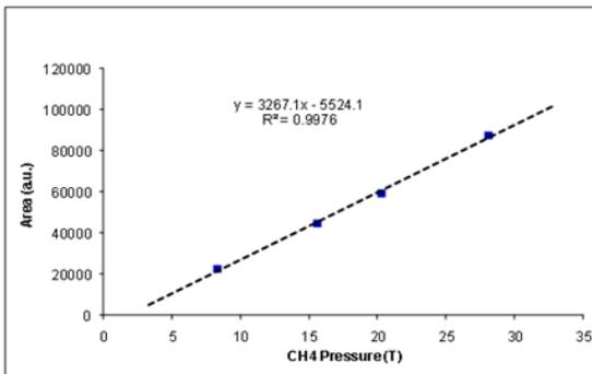
CH<sub>4</sub>calibration: linear relationship of GC responding area vs pressure (with same sampling volume)
