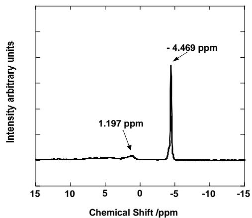
Fig. 1. Solid state MAS  $^1\text{H}$  NMR spectrum of sample prepared using BLP chemicals.
