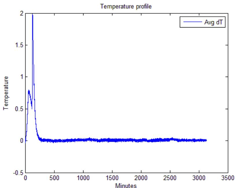
Figure 7: Change in water coolant temperature of heat run for  $\text{MgFe}_2\text{O}_3$  on 4/9/09
