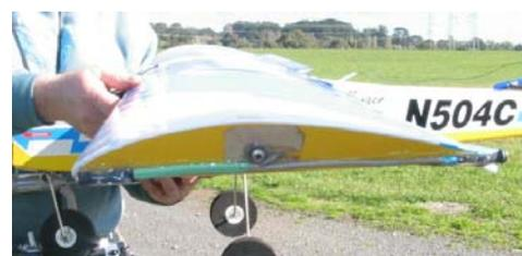
Figure 6. Fixed wingtip sensors
