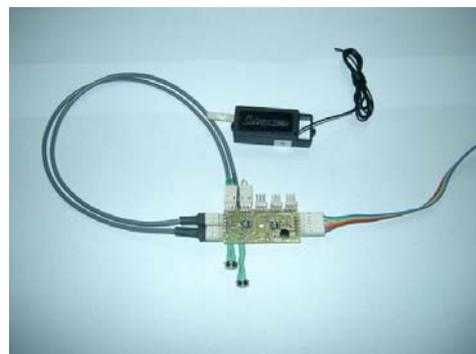
Figure 13. Infrared analog section and RC receiver
