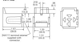
Connector For Use With VF4-2\_\_\_\_ or VF4-5\_\_\_\_ Relays With Shrouded Dust Cover (order terminals separately) VCF4-1003
