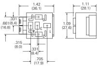
Connector For Use With VF4-3\_\_\_\_ or VF4-6\_\_\_\_ Relays With Weatherproof Cover
