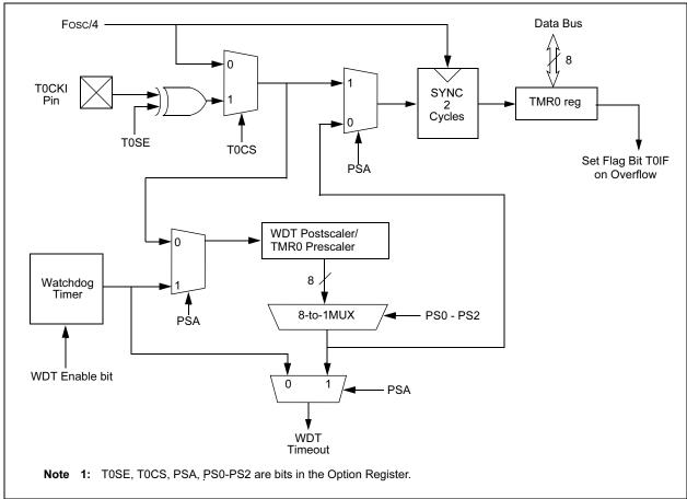
FIGURE 6-1: BLOCK DIAGRAM OF THE TIMER0/WDT
