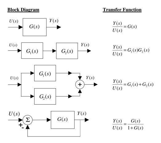
*Transfer functions are ratios of polynomials in 's'*. From the above block diagrams, it can be seen that transfer functions can be made up of a combination of other transfer functions. Thus, in general, transfer functions are ratios of polynomials in 's' as illustrated in the following example. Suppose
