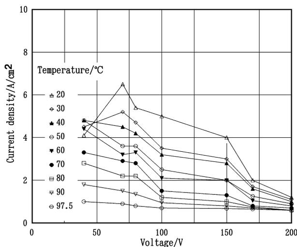
Fig. 3. Typical relationship among voltage, current density and temperature when the cathode was electrolyzed in a 0.2 M  $\text{K}_2\text{CO}_3$  in light water.
