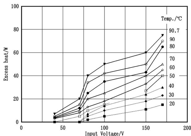
Fig. 7. Effect of the electrolyte temperature on the relationships between heat production and input voltage.
