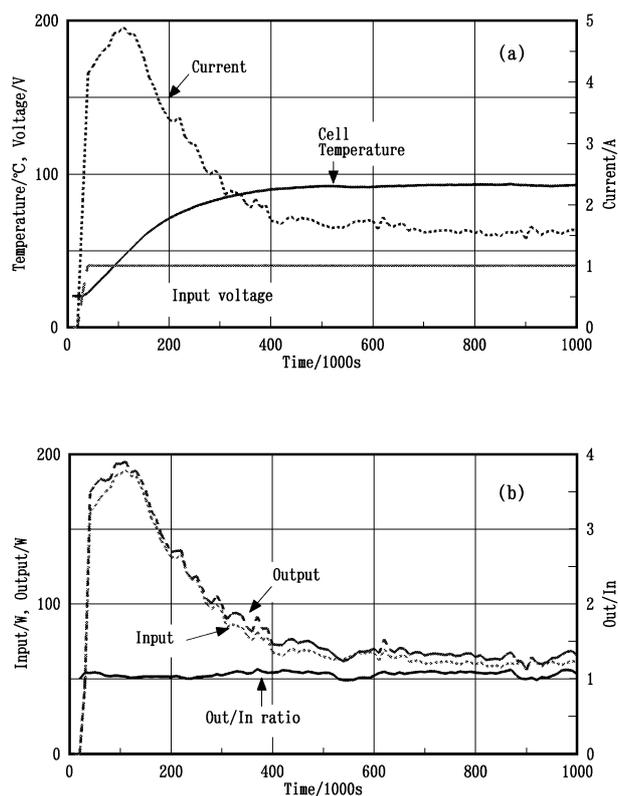
Fig. 4. Measurement of the heat balance for input and output during the ordinary hydrogen production reaction.
