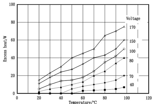
Fig. 8. Effect of the voltage on the relationships between heat production and electrolyte temperature.
