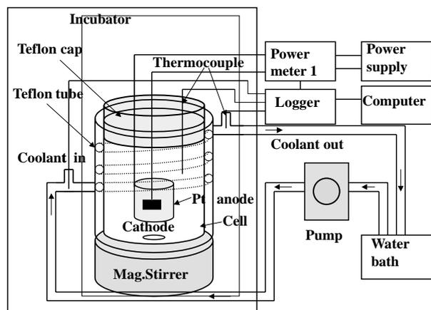
Fig. 1. Schematic of heat measurement apparatus. The method is a combination of open cell isoparabolic calorimetry and flow calorimetry.
