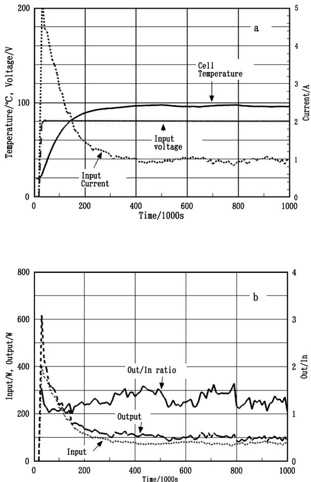
Fig. 5. Result of current density, temperature and the heat balance at 80 V of cathodic electrolysis.
