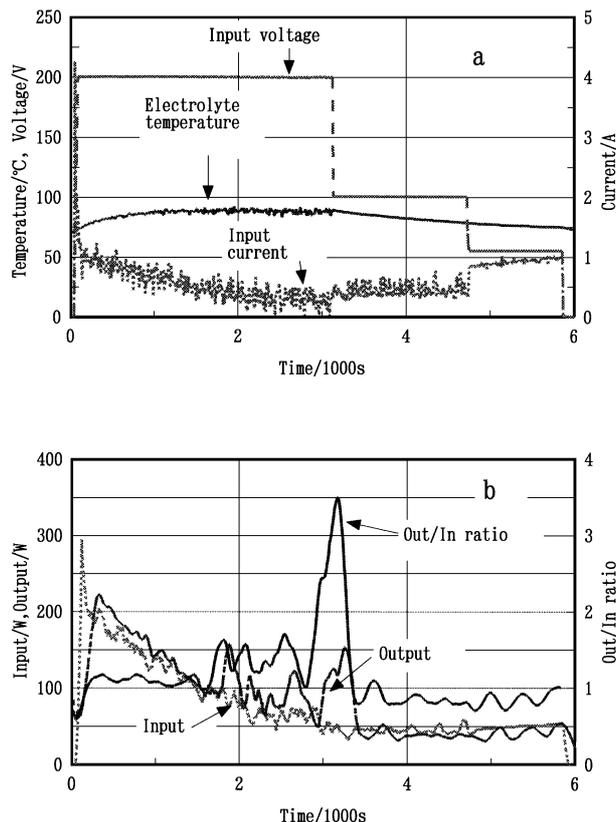
Fig. 6. Result of current density, temperature and heat balance at 200, 100 and 60 V of plasma electrolysis.
