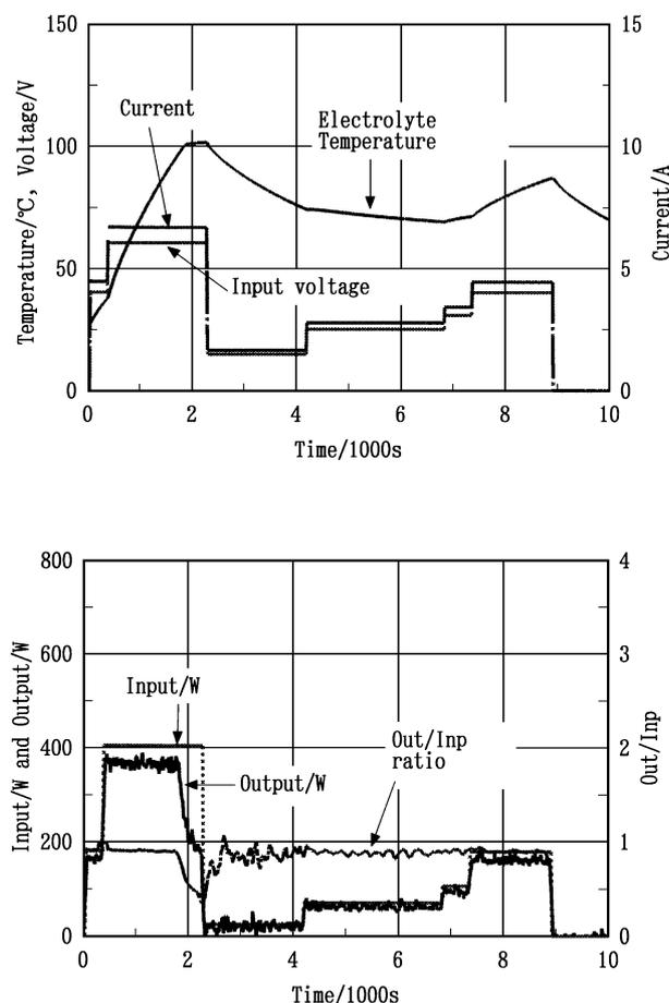
Fig. 2. Result of heat recovery calibration obtained by an electric heater.
