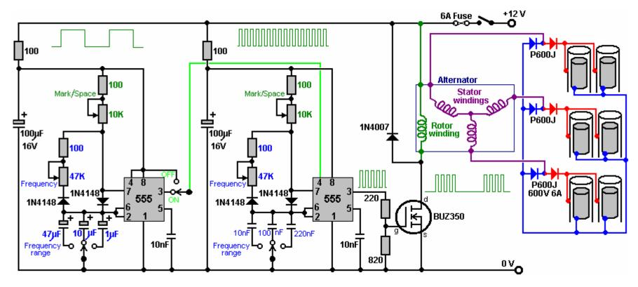
In this rather unusual circuit the rotor winding of an alternator is pulsed via an oscillator circuit which has variable frequency and variable Mark/Space ratio. The oscillator circuit has a degree of supply de-coupling by the 100 ohm resistor feeding the 100 microfarad capacitor. This is to reduce voltage ripple coming along the +12 volt supply line, caused by the current pulses through the rotor winding.
