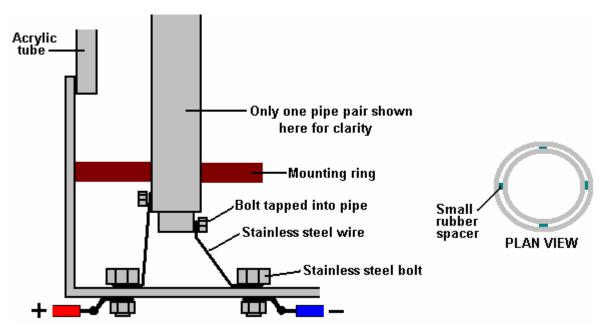
The bolts tapped into the inner tubes should be on the inside and the bottom of the two tubes aligned in spite of them being spread out as shown above. The diagram shows the inner connection on the outside, only for clarity. The bolts going through the base of the unit should be tapped in to give a tight fit and they should be sealed with Sikaflex bonding agent or some similar waterproofing material.
