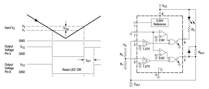
The above figure shows the MC34161 configured as a microprocessor reset with a time delay. Channel 2 monitors input voltage  $V_S$  while channel 1 performs the time delay function. As the input voltage decreases towards ground, the output of channel 2 quickly discharges  $C_{DLY}$  when  $V_S$  falls below  $V_1$ . As the input voltage increases from ground, the output of channel 2 allows  $R_{DLY}$  to charge  $C_{DLY}$  when  $V_S$  exceeds  $V_2$ .
