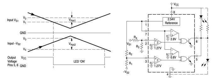
The above figure shows the MC34161 configured as a positive and negative undervoltage detector. As the input voltage decreases toward ground, the LED will turn 'ON' when either  $V_{S1}$  falls below  $V_1$ , or  $-V_{S2}$  falls below  $V_3$ . With the dashed line output connection, the circuit becomes a positive and negative overvoltage detector. As the input voltage increases from the ground, the LED will turn 'ON' when either  $V_{S1}$  exceeds  $V_2$ , or  $-V_{S1}$  exceeds  $V_1$ .
