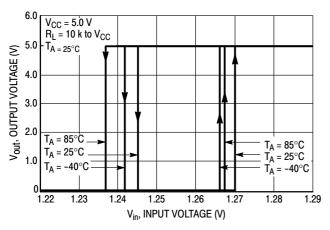
Figure 2. Comparator Input Threshold Voltage
