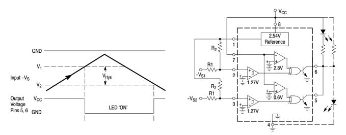
The above figure shows the MC34161 configured as a dual negative undervoltage detector. As the input voltage decreases towards ground, the LED will turn 'ON' when  $-V_{S1}$  or  $-V_{S2}$  falls below V<sub>1</sub>. With the dashed line output connection, the circuit becomes a dual negative overvoltage detector. As the input voltage increases from ground, the LED will turn 'ON' when  $-V_{S1}$  or  $-V_{S2}$  exceeds V<sub>2</sub>.
