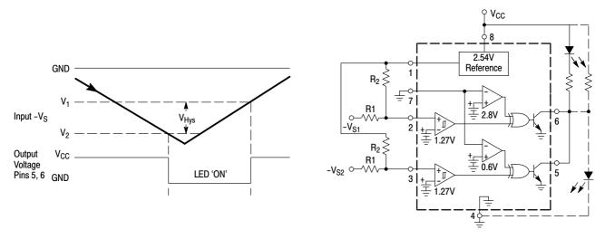
The above figure shows the MC34161 configured as a dual negative overvoltage detector. As the input voltage increases from ground, the LED will turn 'ON' when  $-V_{S1}$  or  $-V_{S2}$  exceeds  $V_2$ . With the dashed line output connection, the circuit becomes a dual negative undervoltage detector. As the input voltage decreases from the peak towards ground, the LED will turn 'ON' when  $-V_{S1}$  or  $-V_{S2}$  falls below  $V_1$ .
