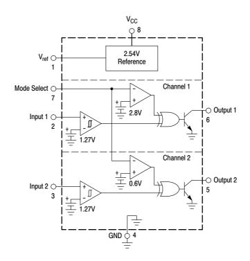
Figure 14. MC34161 Representative Block Diagram
