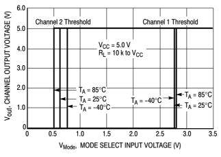
Figure 6. Mode Select Thresholds
