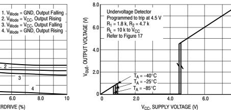
Figure 5. Output Voltage versus Supply Voltage
