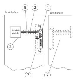
The antenna is of a quarter wave type and is dependent on the groundplane area to complete the antenna function. The antenna performance is also dependent on the size of the groundplane.
