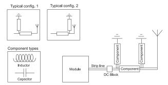
The matching network has to be individually designed using one, two or three components.
