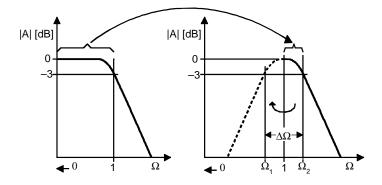
Figure 16-31. Low-Pass to Band-Pass Transition
