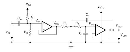
Figure 16-48. Biasing a Sallen-Key Low-Pass
