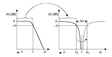
Figure 16-36. Low-Pass to Band-Rejection Transition
