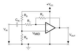
Figure 16–47. Single-Supply Filter Circuit
