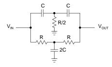
Figure 16-37. Passive Twin-T Filter
