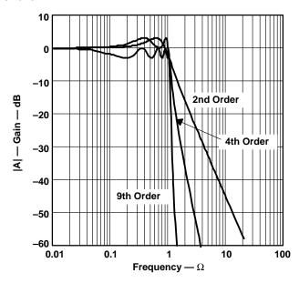
Figure 16-6. Gain Responses of Tschebyscheff Low-Pass Filters
