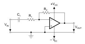
Figure 16-46. Dual-Supply Filter Circuit
