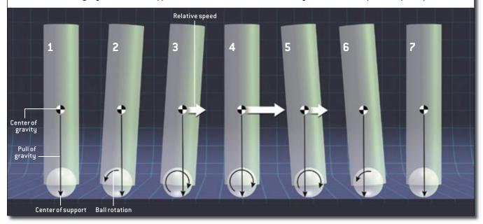
zero in each direction, while minimizing the actions needed to do so. When its objective is to go from one place to another, the control policy automatically institutes a retrograde ball rotation to establish a body tilt, allowing it to accelerate forward. As the goal position is approached, the ball automatically speeds up to reverse the tilt and bring the ballbot to rest [see box above].
