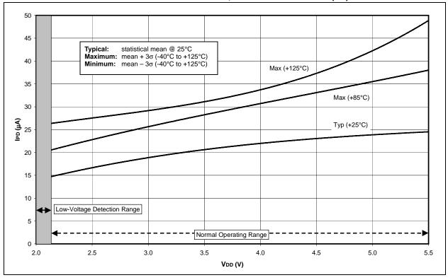
FIGURE 23-32:  $\triangle$ IPD BOR vs. VDD, -40°C TO +125°C SLEEP MODE, BORV1:BORV0 = 11 (2V)
