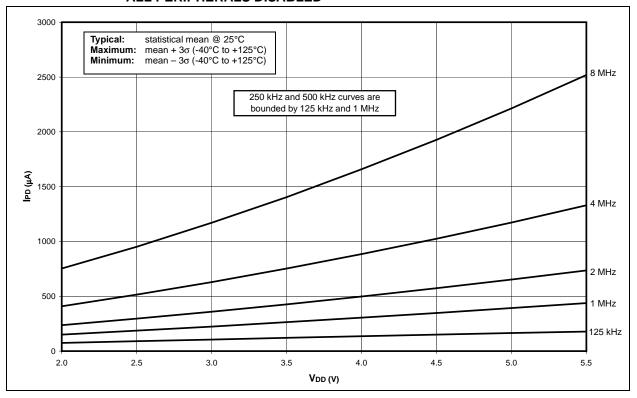
FIGURE 23-16: MAXIMUM IPD vs. VDD (-40°C TO +125°C), 125 kHz TO 8 MHz RC\_RUN MODE, ALL PERIPHERALS DISABLED
