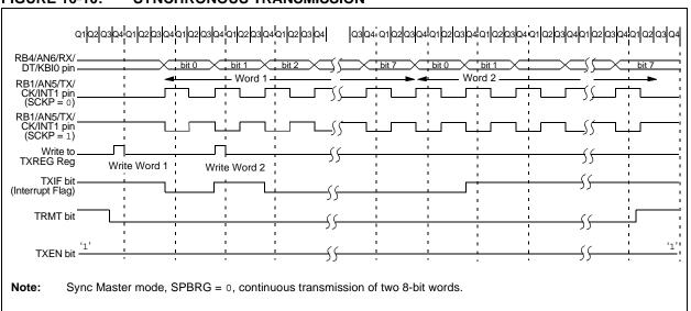
FIGURE 16-11: SYNCHRONOUS TRANSMISSION (THROUGH TXEN)
