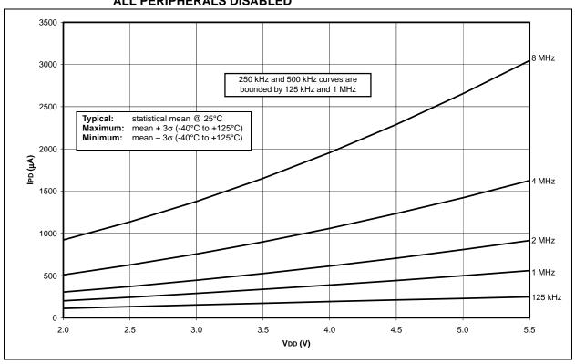
FIGURE 23-17: TYPICAL AND MAXIMUM IPD vs. VDD (-40°C TO +125°C), 31.25 kHz RC\_RUN MODE, ALL PERIPHERALS DISABLED
