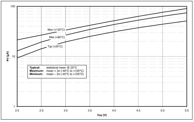
FIGURE 23-18: TYPICAL IPD vs. VDD (+25°C), 125 kHz TO 8 MHz RC\_IDLE MODE, ALL PERIPHERALS DISABLED
