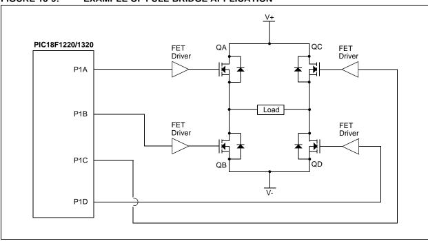
FIGURE 15-9: EXAMPLE OF FULL-BRIDGE APPLICATION
