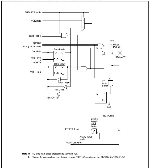
FIGURE 10-8: BLOCK DIAGRAM OF RB1/AN5/TX/CK/INT1 PIN
