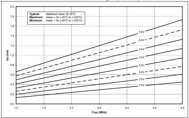
FIGURE 23-5: MAXIMUM IDD vs. FOSC OVER VDD PRI\_RUN, EC MODE, -40°C TO +125°C
