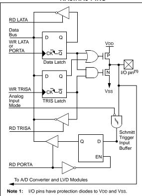
FIGURE 10-3: BLOCK DIAGRAM OF OSC2/CLKO/RA6 PIN
