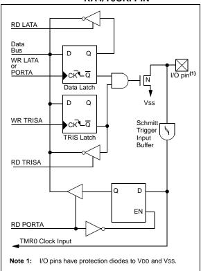
FIGURE 10-5: BLOCK DIAGRAM OF OSC1/CLKI/RA7 PIN
