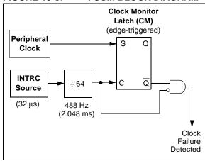
Clock failure is tested for on the falling edge of the sample clock. If a sample clock falling edge occurs while CM is still set, a clock failure has been detected (Figure 19-4). This causes the following:
