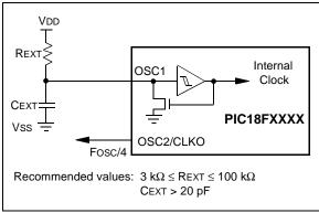
The RCIO Oscillator mode (Figure 2-7) functions like the RC mode, except that the OSC2 pin becomes an additional general purpose I/O pin. The I/O pin becomes bit 6 of PORTA (RA6).
