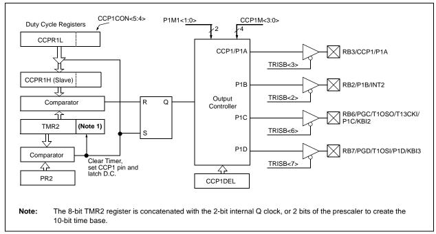
FIGURE 15-4: PWM OUTPUT RELATIONSHIPS (ACTIVE-HIGH STATE)
