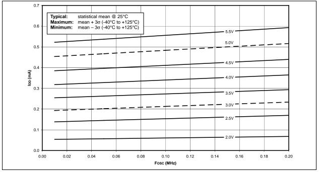
FIGURE 23-3: MAXIMUM IDD vs. Fosc OVER VDD PRI\_RUN, EC MODE, -40°C TO +125°C
