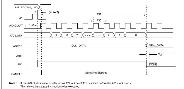
2: This is a minimal RC delay (typically 100 ns), which also disconnects the holding capacitor from the analog input.
