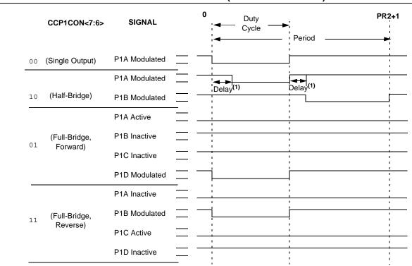
FIGURE 15-5: PWM OUTPUT RELATIONSHIPS (ACTIVE-LOW STATE)
