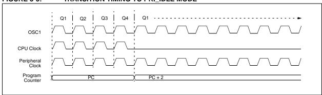
FIGURE 3-4: TRANSITION TIMING FOR WAKE FROM PRI IDLE MODE
