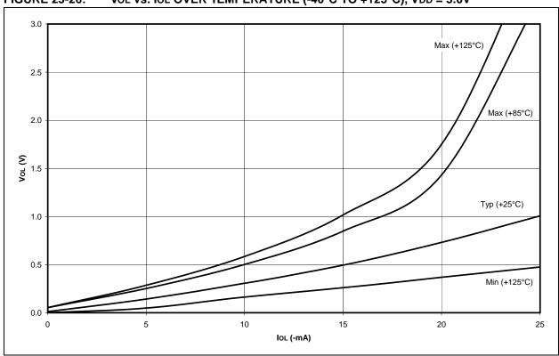
FIGURE 23-27: Vol vs. Iol OVER TEMPERATURE (-40°C TO +125°C), VDD = 5.0V
