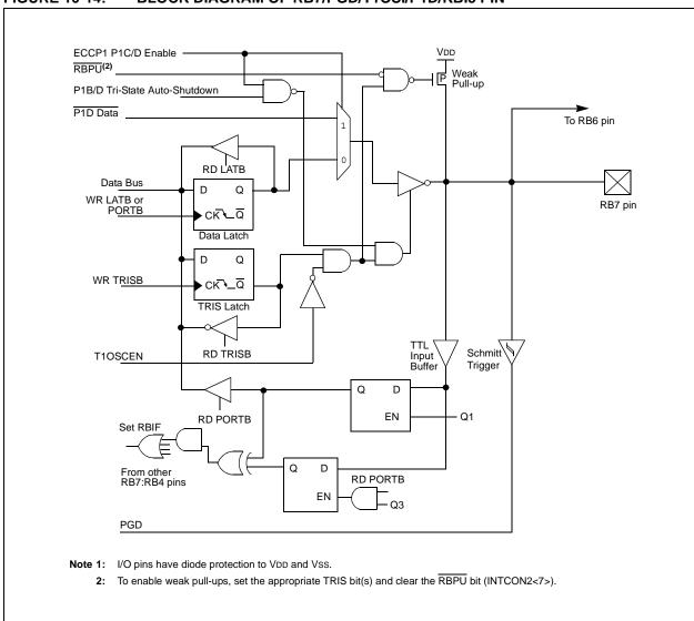
FIGURE 10-14: BLOCK DIAGRAM OF RB7/PGD/T10SI/P1D/KBI3 PIN
