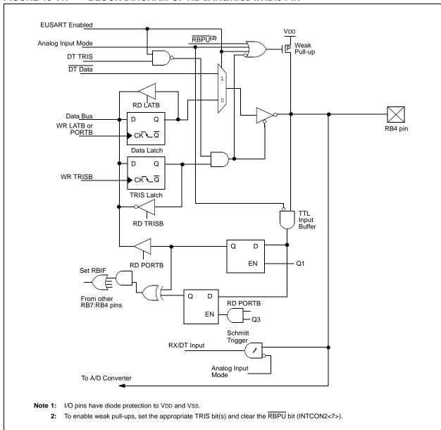
FIGURE 10-11: BLOCK DIAGRAM OF RB4/AN6/RX/DT/KBI0 PIN
