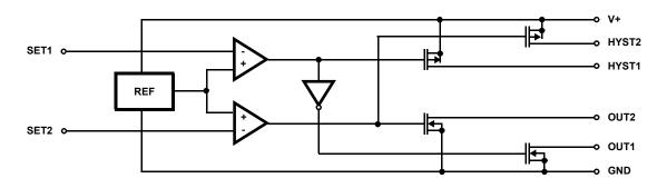
$\label{eq:second} \begin{array}{l} \mbox{CONDITIONS} \mbox{ (Note 5)} \\ V_{SET1} > 1.3V, \mbox{ OUT1} \mbox{ Switch ON}, \mbox{ HYST1} \mbox{ Switch OFF} \\ V_{SET2} > 1.3V, \mbox{ OUT2} \mbox{ Switch OFF}, \mbox{ HYST2} \mbox{ Switch OFF} \\ V_{SET2} < 1.3V, \mbox{ OUT2} \mbox{ Switch ON}, \mbox{ HYST2} \mbox{ Switch OFF} \end{array}$
