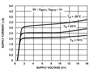
FIGURE 6. SUPPLY CURRENT AS A FUNCTION OF SUPPLY VOLTAGE
