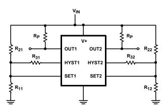
FIGURE 11. AN ALTERNATIVE HYSTERESIS CIRCUIT
