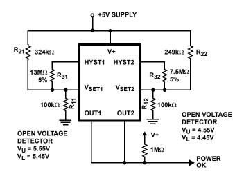
FIGURE 12. FAULT MONITOR FOR A SINGLE SUPPLY
