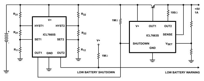
FIGURE 14. LOW BATTERY WARNING AND LOW BATTERY DISCONNECT
