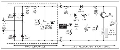
and sounds the buzzer (alarm) to give a warning of the power-failure.
