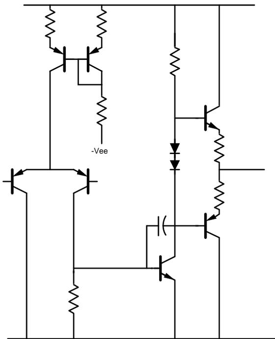
Here we have simplified the circuit by eliminating the constant-current loads. This will reduce the gain and make the amplifier harder to bias right.
