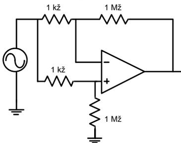
If the resistors are well-matched (take the time to find resistors accurate to 1% or better before testing), then the circuit gain will be about  $(2000)A_{CM}/A_D$
