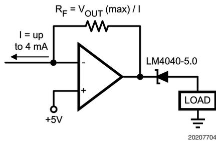
**FIGURE 4. Current-to-voltage converter with offset correction.**
