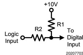
**FIGURE 3. Simple digital input level shifting circuit**
