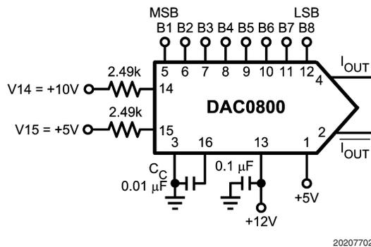
**FIGURE 2. Positive only supply circuit for the DAC0800**
