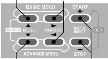
To PMIX-2 These keys are used to move around in the PMIX-1 menu
