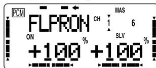
Connect the right aileron servo to receiver CH1 and the left aileron servo to receiver CH6.
