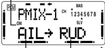
Master channel (control that applies mixing) Slave channel (channel which receives mixing)
