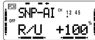
We recommend that you activate the safety switch. This stops your model from snap rolling if the landing gear are not retracted, so you don't accidentally snap while taking off or landing.
