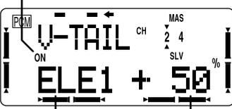
2. Set elevator travel for CH2 servo with the (+)/(-) keys. Repeat for:
