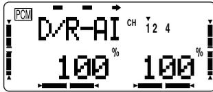
Aileron Dual Rates: adjust the aileron travel to roughly 7/16" (11 mm). You may also wish to adjust EXP so that its rate is -20 to -30% to soften things around neutral.
