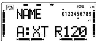
3. Enter the Parameter (PARA, p. 31) menu by pressing the down MODE key twice. Use the left (<) CURSOR key to select the model type (TYP) function and verify that ACRO (aircraft) is selected. (If it isn't, select ACRO by pressing the plus or minus DATA INPUT keys until it appears, then pressing both DATA INPUT keys to select it.)
