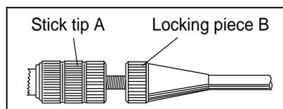
Next, move the locking piece B up or down (to lengthen or shorten). When the length feels comfortable, lock the position by turning locking piece B counterclockwise.
