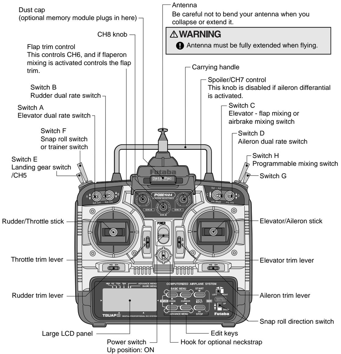
This figure shows the default assignments for a Mode 2 system as supplied by the factory. You can change many of the switch positions or functions by selecting a new position within the setting menu for the function you wish to move.
