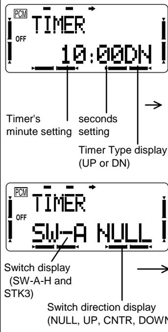
The diagram shows two states of the 8UA timer display. The top display shows '10:00DN' with labels for 'Timer's minute setting' (the '10'), 'seconds setting' (the ':00'), and 'Timer Type display (UP or DN)' (the 'DN'). The bottom display shows 'SW-A NULL' with labels for 'Switch display (SW-A-H and STK3)' (the 'SW-A') and 'Switch direction display (NULL, UP, CNTR, DOWN)' (the 'NULL').
