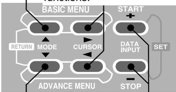
These keys are used to move through the five submenus in the OFST1 & OFST2 functions.
