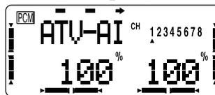
Aileron settings: the left and right aileron travel should be limited to roughly 9/16" (14-15 mm). If necessary, adjust CH1 and CH6 with the ATV function. Choose a location on the servo arm so that the throw is adjusted in the 90-100% range.
