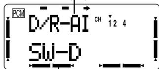
D/R switch display (SW-A, SW-B, SW-D, SW-E for helicopters, STK-1, STK-2, STK-3, STK-4)
