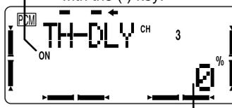
Turn the TH-DLY function ON by pressing the (+) key ("ON" displayed). Turn off (INH) the function with the (-) key.
