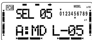
2. Press the right (>) CURSOR key twice to get to the model name function (NAME, p. 37). Use the CURSOR and DATA INPUT keys to spell out the name that you wish to appear on the screen, one letter at a time.
