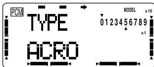
**WARNING:** selecting a different model type will erase the settings in the model memory. BE SURE you're in the correct model memory before selecting a new model type.
