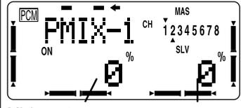
Mixing rate (left or up)      Mixing rate (right or down)
