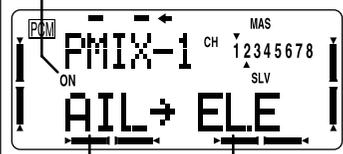
Master channel (control that applies mixing)      Slave channel (channel which receives mixing)
