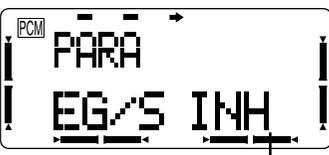
Current setting display (one of CH5, CH7, CH8 or INH). The default setting is INH (inhibited).
