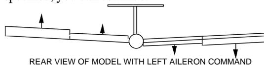
Reverse any of CH1, 5, 6, and 7 by moving to the appropriate channel number with the right or left CURSOR keys, then pressing the minus (-) or Plus (+) DATA INPUT key to reverse or unreverse the channel. Be sure you get the aileron response in the picture.
