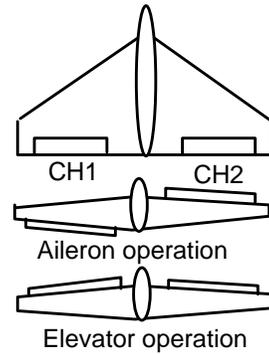
**NOTE:** The elevon, flaperon, aileron differential, and ailevator functions cannot be activated simultaneously. The function activated last has priority.
