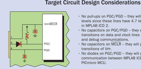
No pull-ups on PGC/PGD – they will divide the voltage levels since these lines have 4.7 k $\Omega$  pull-down resistors in MPLAB ICD 2.
