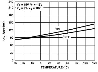
FIGURE 9. SWITCHING TIME vs TEMPERATURE
