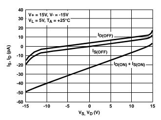
FIGURE 10. LEAKAGE CURRENTS vs ANALOG VOLTAGE
