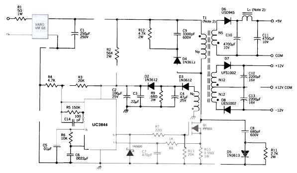
Fig 5 - 25 W Off-Line Flyback Regulator
