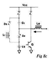
rise of voltage across the switch. The two capacitors are effectively operating in parallel even though one is charging and the other is discharging.
