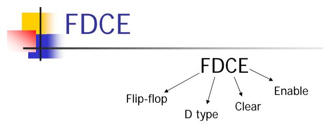
So it's a D flip-flop with Clear and Enable signals, and Clear has priority over Enable.
