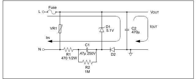
Figure 10 shows a capacitive power supply with several UL considerations designed in. A fuse is added to protect the circuit during an over-current condition. Adding R2 in parallel with C1 creates a filter that will attenuate EMI from traveling back onto the line. A varistor, or MOV, provides transient protection.
