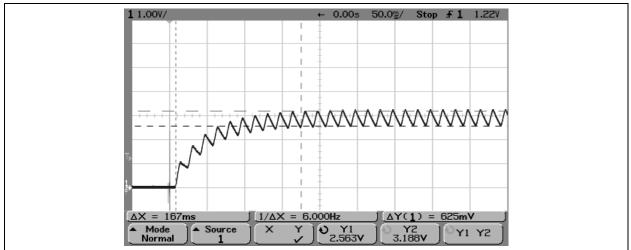
When working with an 60 Hz AC source, it is often desirable to know when the line voltage crosses Neutral. The crossing, known as zero-cross, can easily be captured by connecting the node formed by D1, C1 and D2 to an input on the microcontroller. The waveform observed at this node is shown in Figure 9.
