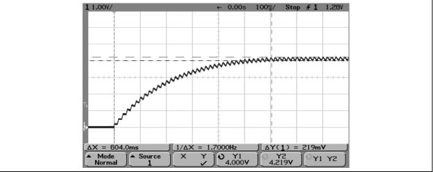
If even more current is demanded from the circuit, the supply will stabilize at a voltage below the desired level. Figure 4, shows an oscilloscope plot of VOUT during the same time frame for a 270 $\Omega$  load. A 270 $\Omega$  load will draw approximately 16 mA with an output voltage of 4.5V. This current cannot be provided by the circuit, therefore, the output voltage is compromised.
