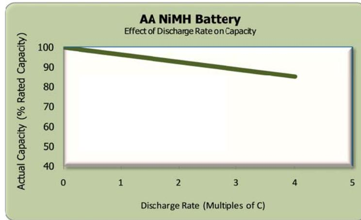
(Fig. 10) Effect of Discharge Rate on Capacity
