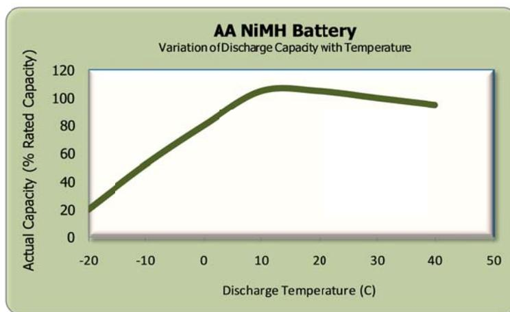
(Fig. 9) Variation of Discharge Capacity with Temperature
