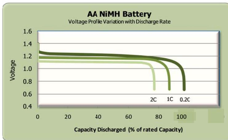
(Fig. 8) Voltage Profile Variation with Discharge Rate
