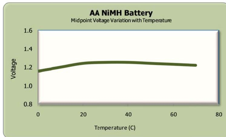
(Fig. 7) Midpoint Voltage Variation with Temperature
