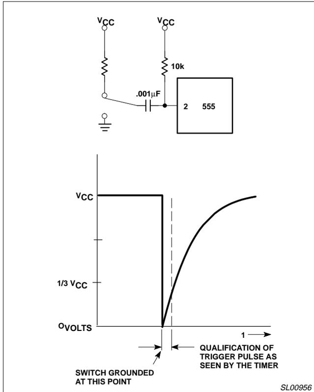
Figure 3. AC Coupling of the Trigger Pulse
