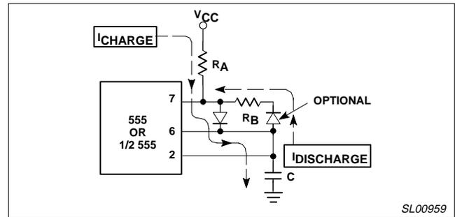
**Figure 6. Method of Achieving Duty Cycles Less Than 50%**
