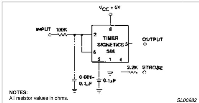
Figure 29. Low Cost Line Receiver
