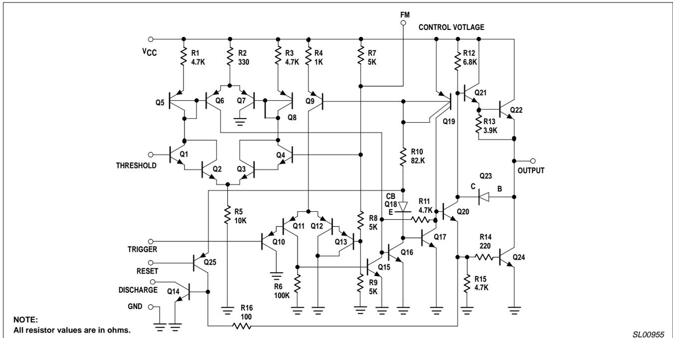
Figure 2. Schematic of 555 or 1/2 556 Dual Timer
