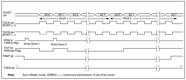
FIGURE 12-11: SYNCHRONOUS TRANSMISSION (THROUGH TXEN)
