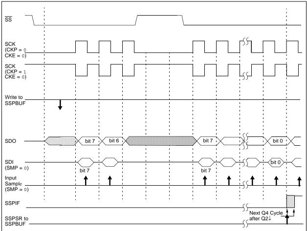
FIGURE 13-4: SPI MODE WAVEFORM (SLAVE MODE WITH CKE = 0)
