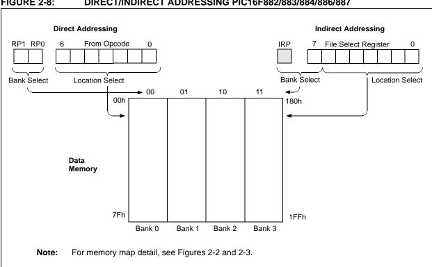
FIGURE 2-8: **DIRECT/INDIRECT ADDRESSING PIC16F882/883/884/886/887**
