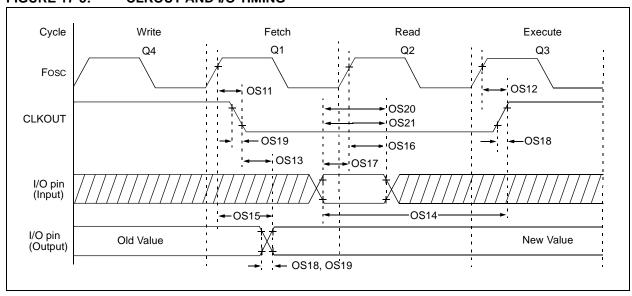
TABLE 17-3: CLKOUT AND I/O TIMING PARAMETERS
