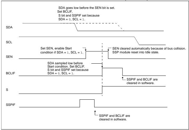
FIGURE 13-22: BUS COLLISION DURING START CONDITION (SCL = 0)
