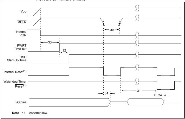
FIGURE 17-7: BROWN-OUT RESET TIMING AND CHARACTERISTICS
