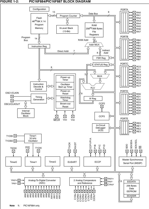
FIGURE 1-2: PIC16F884/PIC16F887 BLOCK DIAGRAM
