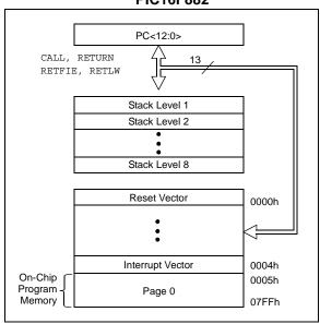
FIGURE 2-2: PROGRAM MEMORY MAP AND STACK FOR THE PIC16F883/PIC16F884
