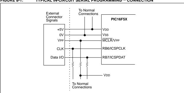
TYPICAL IN-CIRCUIT SERIAL PROGRAMMING™ CONNECTION FIGURE 8-1:
