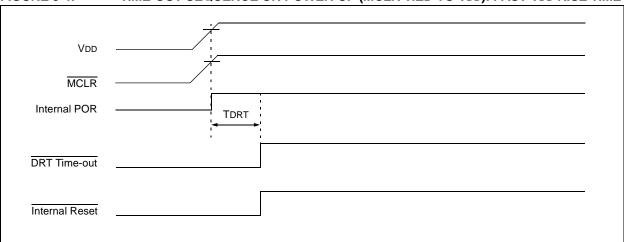
FIGURE 5-5: TIME-OUT SEQUENCE ON POWER-UP (MCLR TIED TO VDD): SLOW VDD RISE TIME
