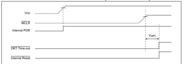
FIGURE 5-4: TIME-OUT SEQUENCE ON POWER-UP (MCLR TIED TO VDD): FAST VDD RISE TIME
