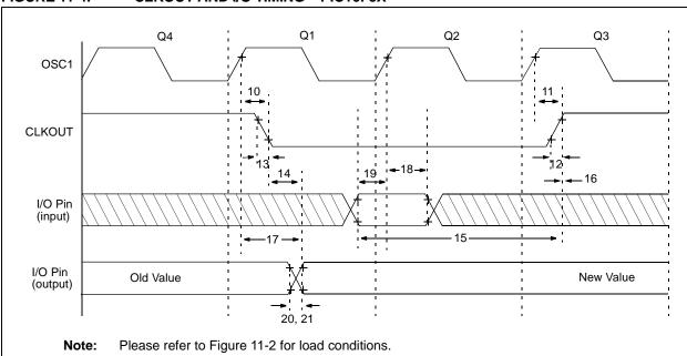
FIGURE 11-4: CLKOUT AND I/O TIMING – PIC16F5X
