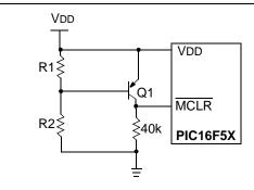
This brown-out circuit is less expensive, although less accurate. Transistor Q1 turns off when VDD is below a certain level such that:
