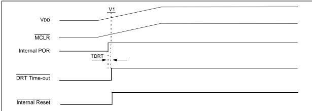
Note: When VDD rises slowly, the TDRT time-out expires long before VDD has reached its final value. In this example, the chip will reset properly if, and only if, V1 ≥ VDD min.
