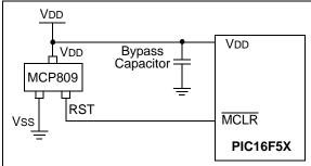
This brown-out protection circuit employs Microchip Technology's MCP809 microcontroller supervisor. The MCP8XX and MCP1XX families of supervisors provide push-pull and open collector outputs with both "active-high and active-low" Reset pins. There are 7 different trip point selections to accommodate 5V and 3V systems.
