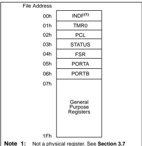
Note 1: Not a physical register. See Section 3.7 "Indirect Data Addressing; INDF and FSR Registers".
