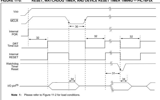
RESET, WATCHDOG TIMER, AND DEVICE RESET TIMER TIMING -- PIC16F5X **FIGURE 11-5:**
