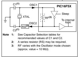
FIGURE 4-2: EXTERNAL CLOCK INPUT OPERATION (HS, XT OR LP OSC CONFIGURATION)
