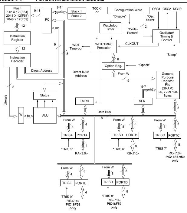
FIGURE 2-1: PIC16F5X SERIES BLOCK DIAGRAM
