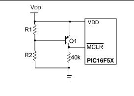
This brown-out circuit is less expensive, although less accurate. Transistor Q1 turns off when VDD is below a certain level such that:
