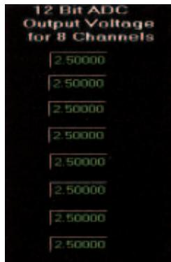
This front-panel view represents a LabView Virtual Instrument for an eight-channel ADC.
