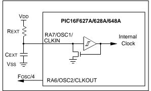
The RC Oscillator mode has two options that control the unused OSC2 pin. The first allows it to be used as a general purpose I/O port. The other configures the pin as an output providing the Fosc signal (internal clock divided by 4) for test or external synchronization purposes.
