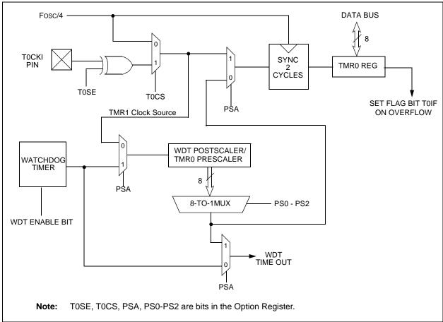
FIGURE 6-1: BLOCK DIAGRAM OF THE TIMER0/WDT
